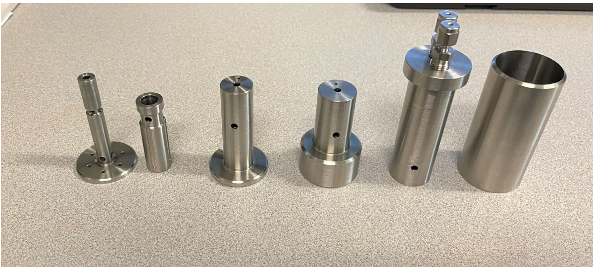
Figure 14. Air piloted actuator assembly components
