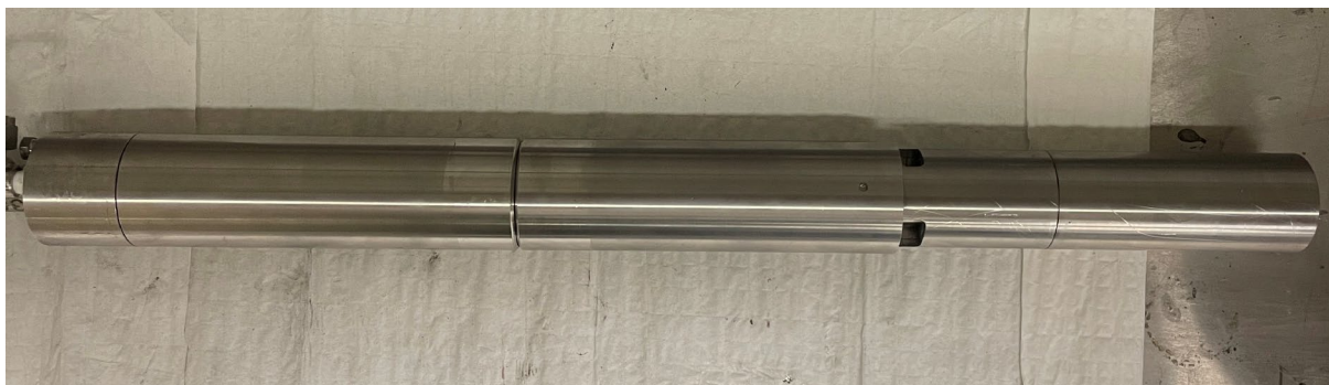
Figure 15. Final assembly of the RT-SEISMIC impulse source module
