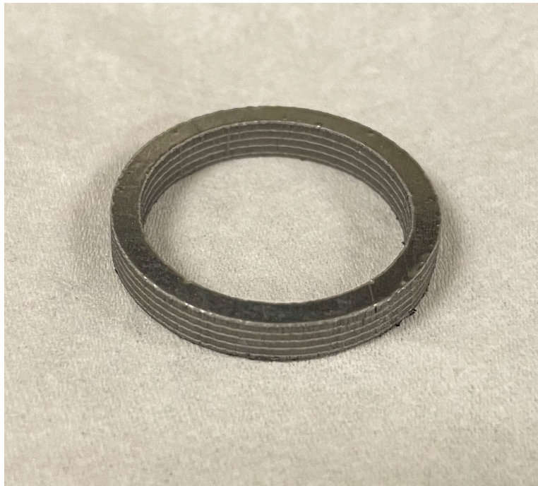
Figure 8. Composite graphite-aluminum seals used for dynamic reciprocating motion of the shuttle assembly
