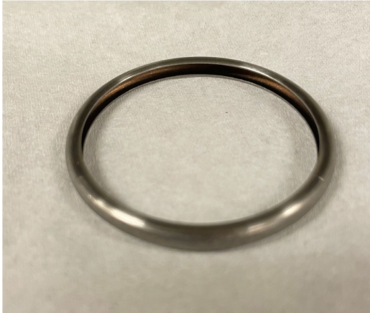
Figure 7. Inconel C-rings used for RT-SEISMIC static seals
