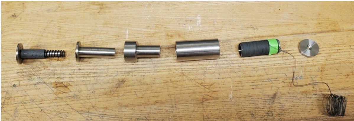
Figure 12. Electromagnetic solenoid actuator that was initially designed for use in the RT-SEISMIC source module
