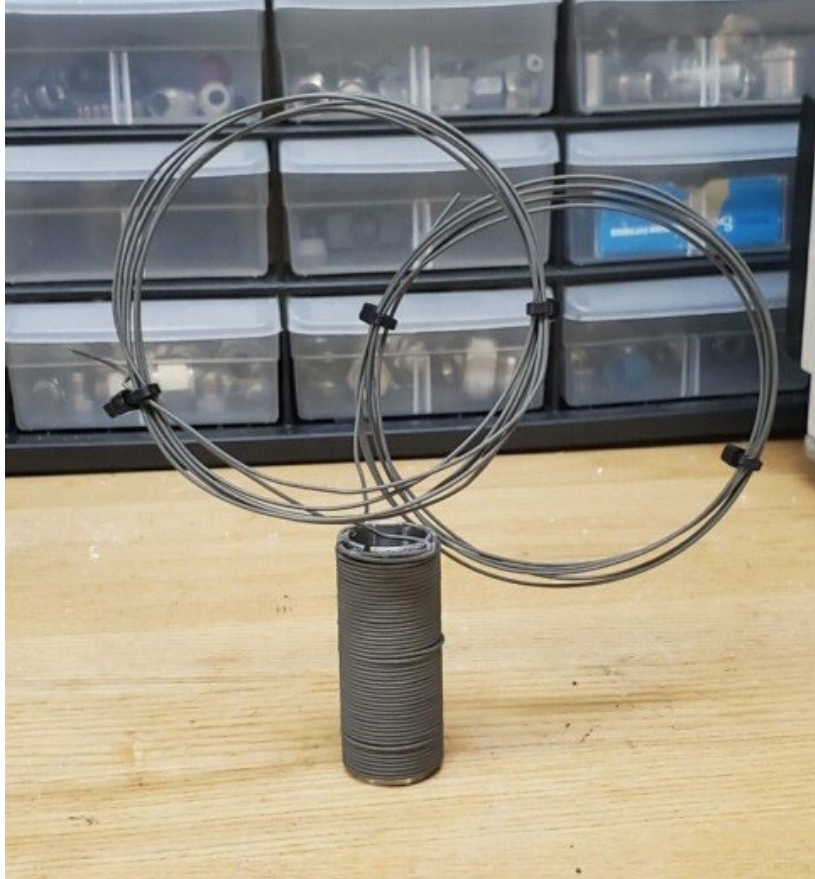
Figure 13. Electromagnetic solenoid winding
