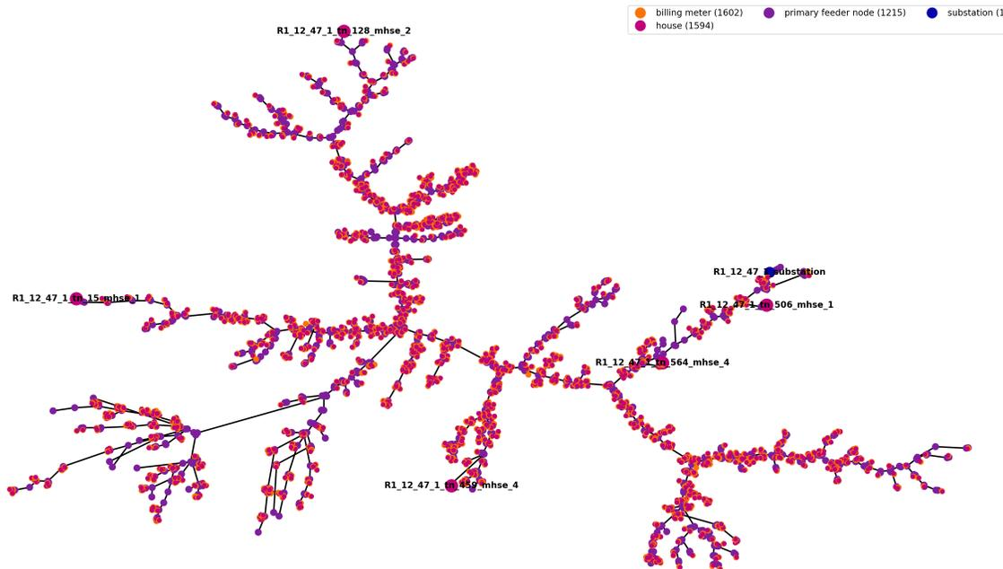
Figure 7: ns-3 network used in this capability demonstration with all billing meters implemented
