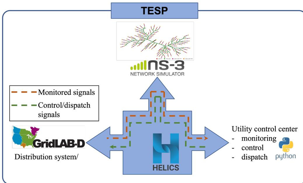
Figure 2: TESP architecture.
