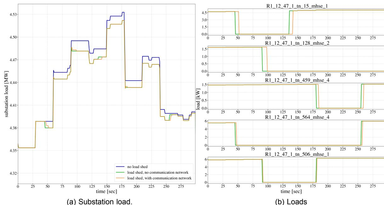
Figure 8: Impacts of communication system latency on load management system performance
