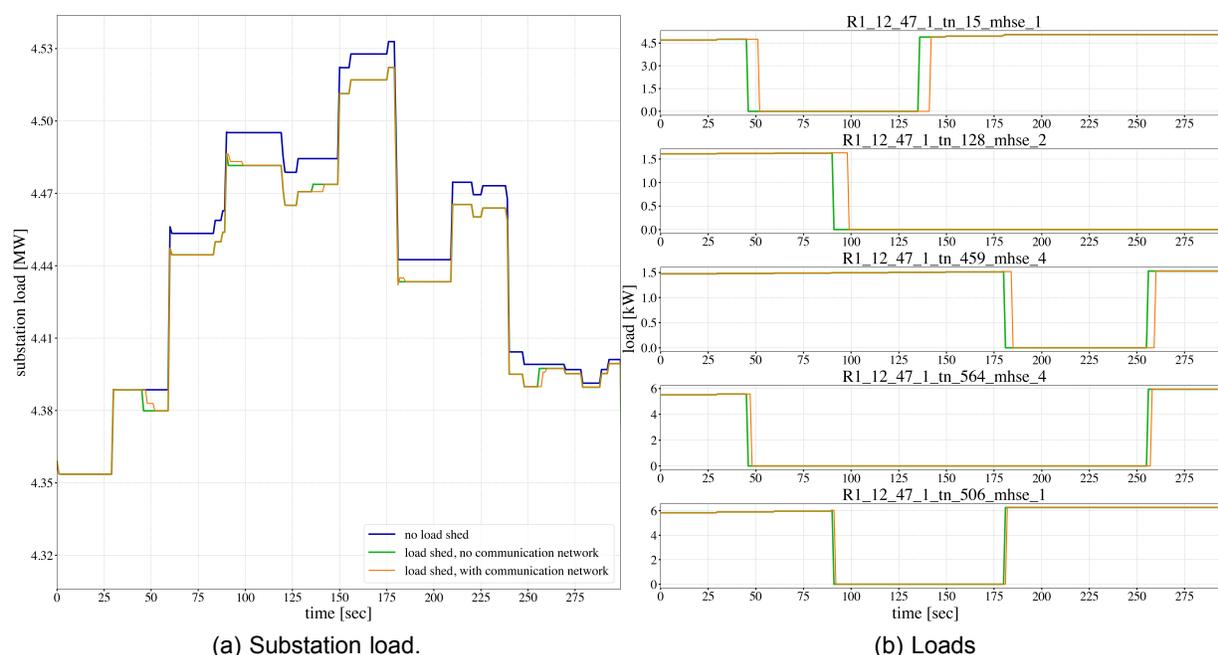
Figure 1: Impacts of communication system latency on load management system performance
