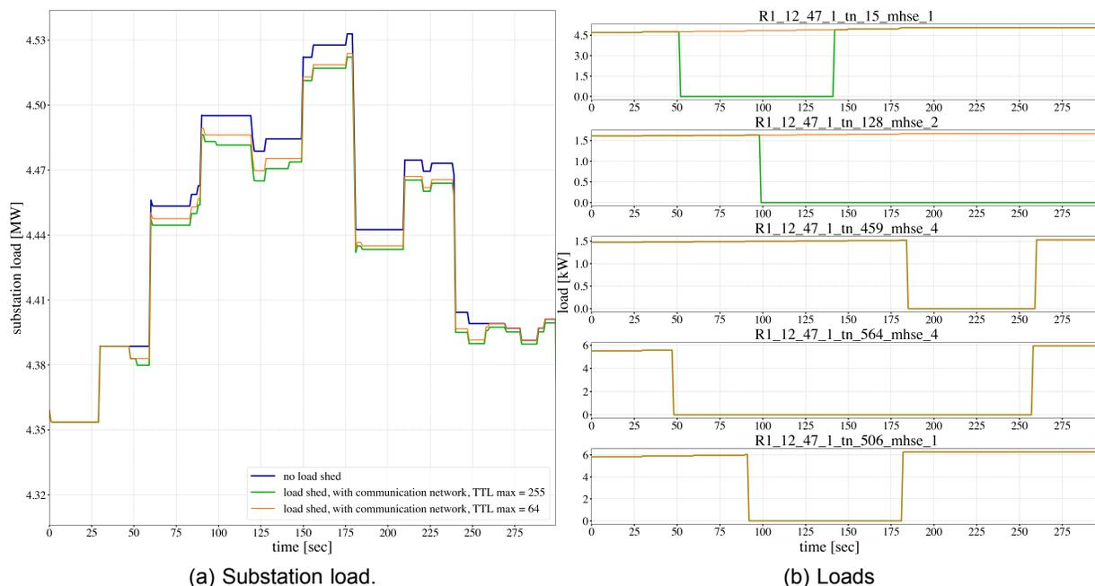
Figure 9: Results showing the impact of packet loss on load curtailment.
