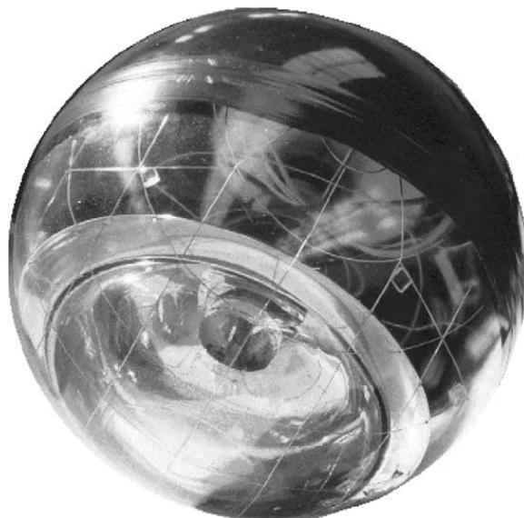
Figure A.12. A photograph of the ANTARES optical module.
