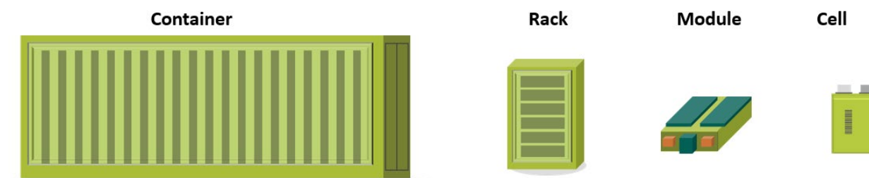
Figure 3. ESS components: from container to cell.
