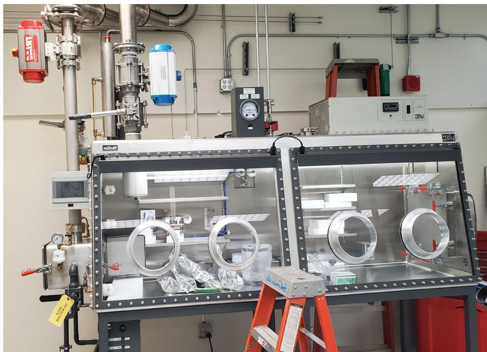
Figure 17. Inert radiological glove box for storage, mixing, and loading of hydroscopic coolant and fuel salts.
