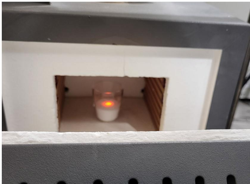
Figure 14: Guiding light from the pyrometer on  $\text{ClNaK5149}$  in the muffle furnace at  $550\text{ }^{\circ}\text{C}$ . Note the use of larger crucibles and the crucibles closer to the pyrometer in this second study, ensuring the guide light (i.e. laser) is well within the crucible and not capturing signal from the crucible wall.
