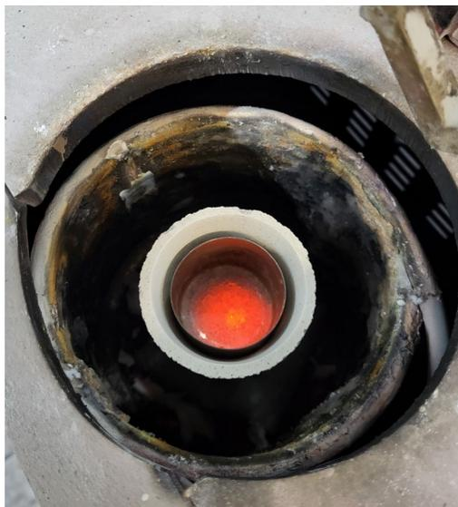
Figure 12. Shows the size of the pyrometer LED size which should be much larger than the incident area of the pyrometer laser.
