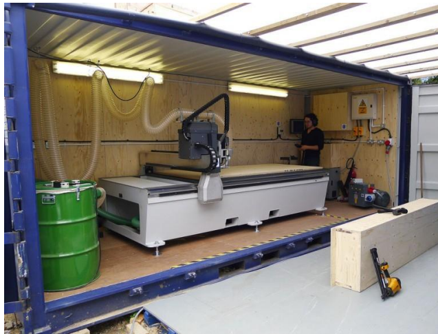
Figure 7. Facit's CNC machine, transported to home sites in a shipping container, cuts customized pieces for homes. (Source: Facit)
