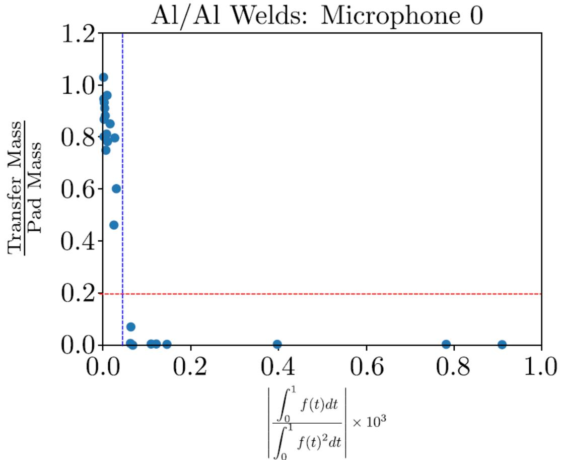
**Figure 2.** Summary plot of mean weight change vs. normalized energy differential for all aluminum-to-aluminum welds. The vertical axis is a proxy for a good weld (higher is better). Red line shows presumed cutoff between good (left of dashed blue line) and bad (right of dashed blue line) welds. Using this cutoff there are zero false positives and zero false negatives. Once qualified, data such as those shown above could be used to produce a bone fide receiver operator curve.
