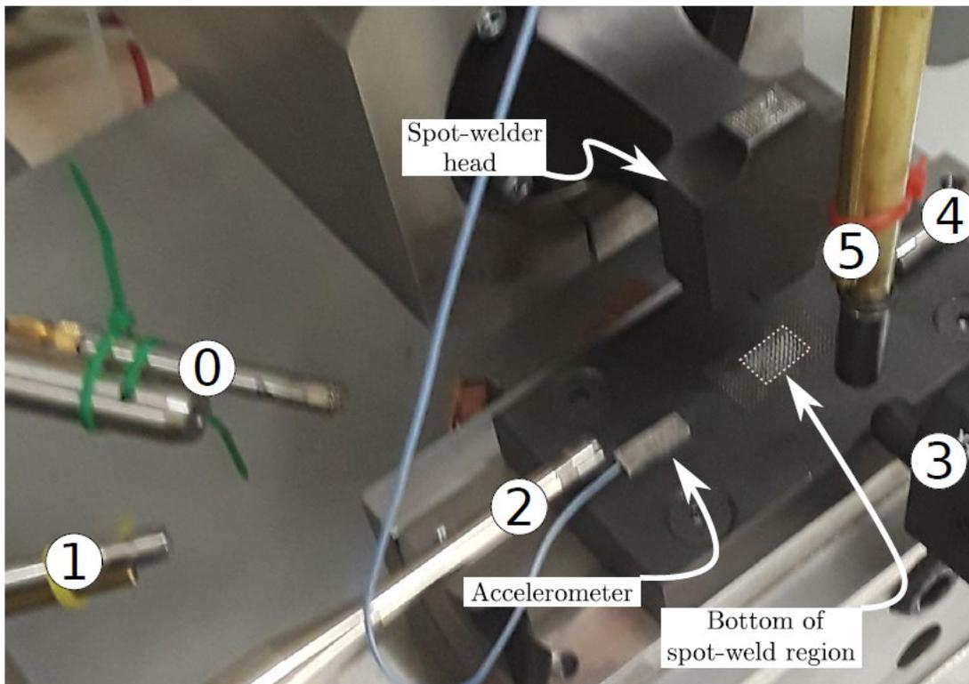
**Figure 1.** Placement of the six microphones used for acquisition of acoustic signatures produced during ultrasonic welding. An accelerometer was mounted on the welder base as an additional source of data (however, not reported in this study). The "passive" area of the bottom spot weld region is also indicated.
