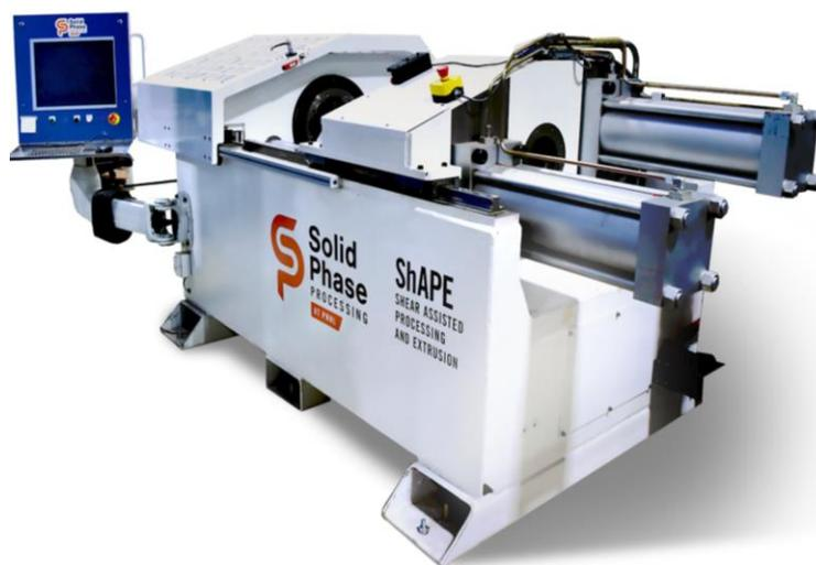
Figure 1: Shear assisted processing and extrusion equipment available at PNNL used for manufacturing lead free brass wires, rods, and tubes in this project.
