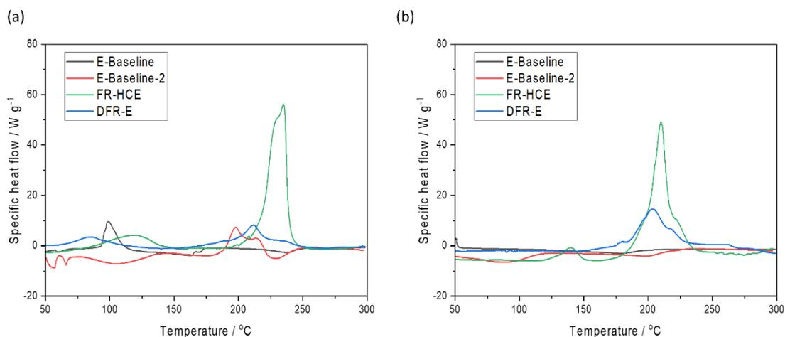
Figure 6. Heat flow of (a) lithiated Gr electrode and (b) delithiated LFP electrode in the presence of the formulated electrolytes. (Obtained with DSC with the temperature increase rate of 10 °C min<sup>-1</sup>).
