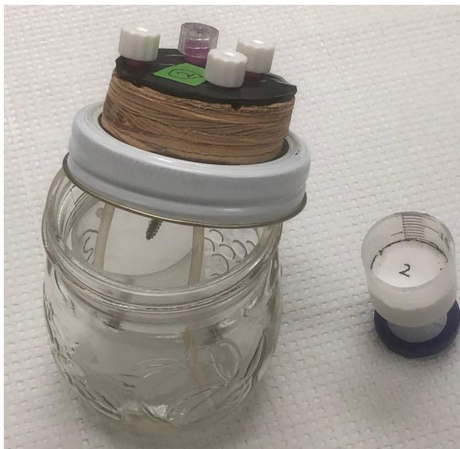
Figure 3. N-release test apparatus. Reaction vessel is on right, and leachate collection vessel is inside the jar. Note fine-bore Teflon tubing connected to sampling ports and used to sample leachate and the  $\text{H}_3\text{BO}_3$  solution outside the leachate collection vessel.
