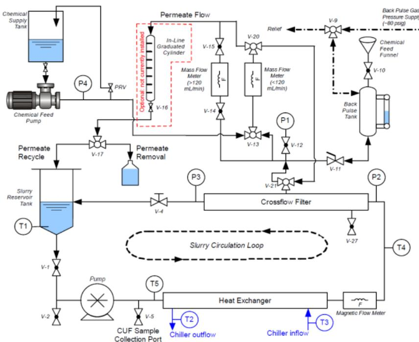
Figure 2 Filter System Piping & Instrumentation Diagram
