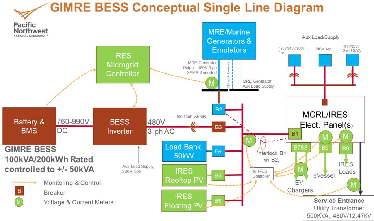
Figure 1-2. Conceptual Overview of BESS and Tidal Generation Electrical Connections
