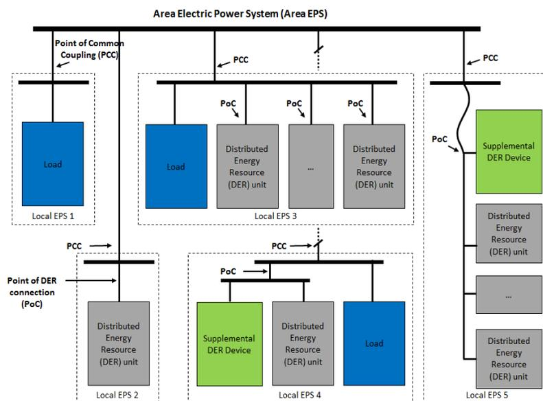
Figure 2-1. IEEE 1547 Interconnection Point of Connection vs Point of Common Coupling
