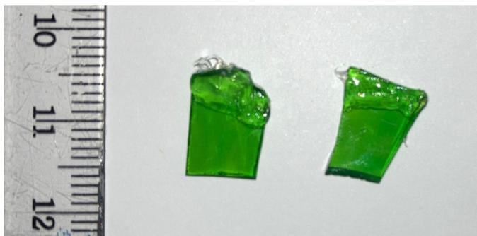
Figure 2-3. Examples of masked coupons before testing. The ruler scale is in centimeters.
