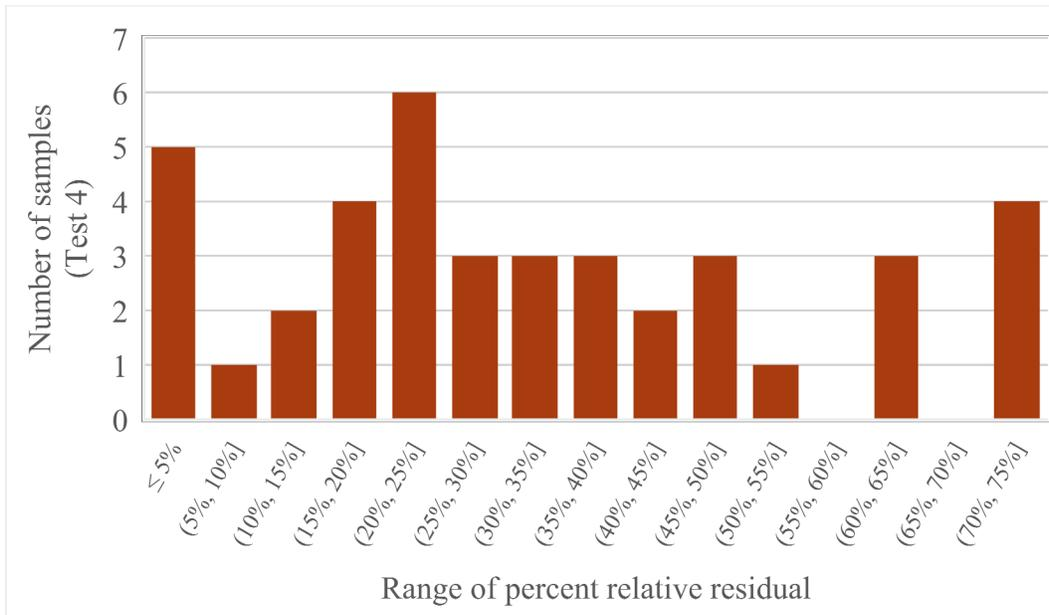
Figure 4-8 – The distribution of percent relative residual values for all Test 4 samples ( $\text{pH}_{(\text{RT})} = 11$ , 70 °C)
