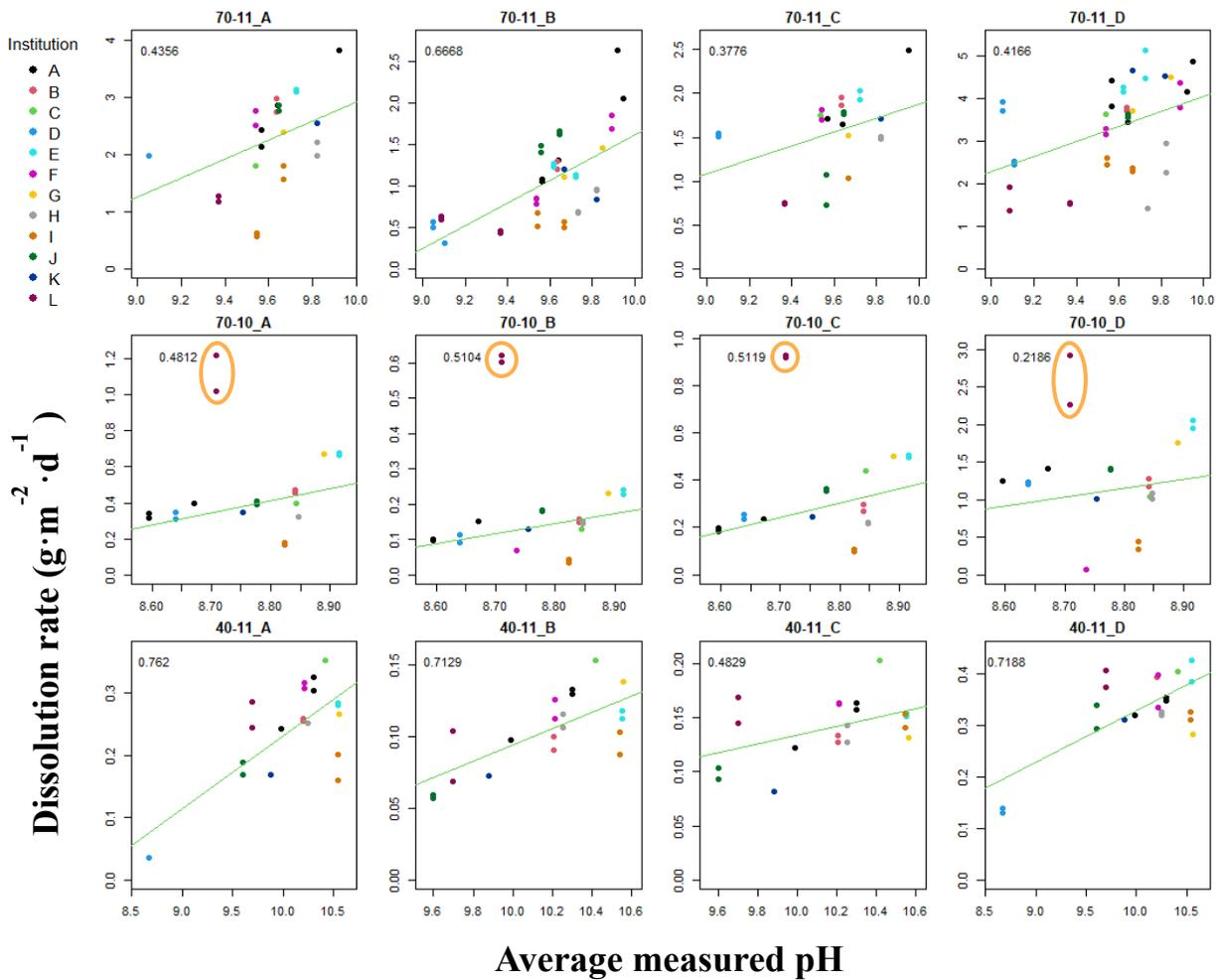
Figure 4-2 - Average dissolution rate as a function of pH for each test in all conditions. For each condition, a linear fit is presented with the R<sup>2</sup> value in the upper left of each plot. Outlier data points from the pH<sub>(RT)</sub> = 10 and 70 °C conditions that were excluded from further analysis are circled in orange.
