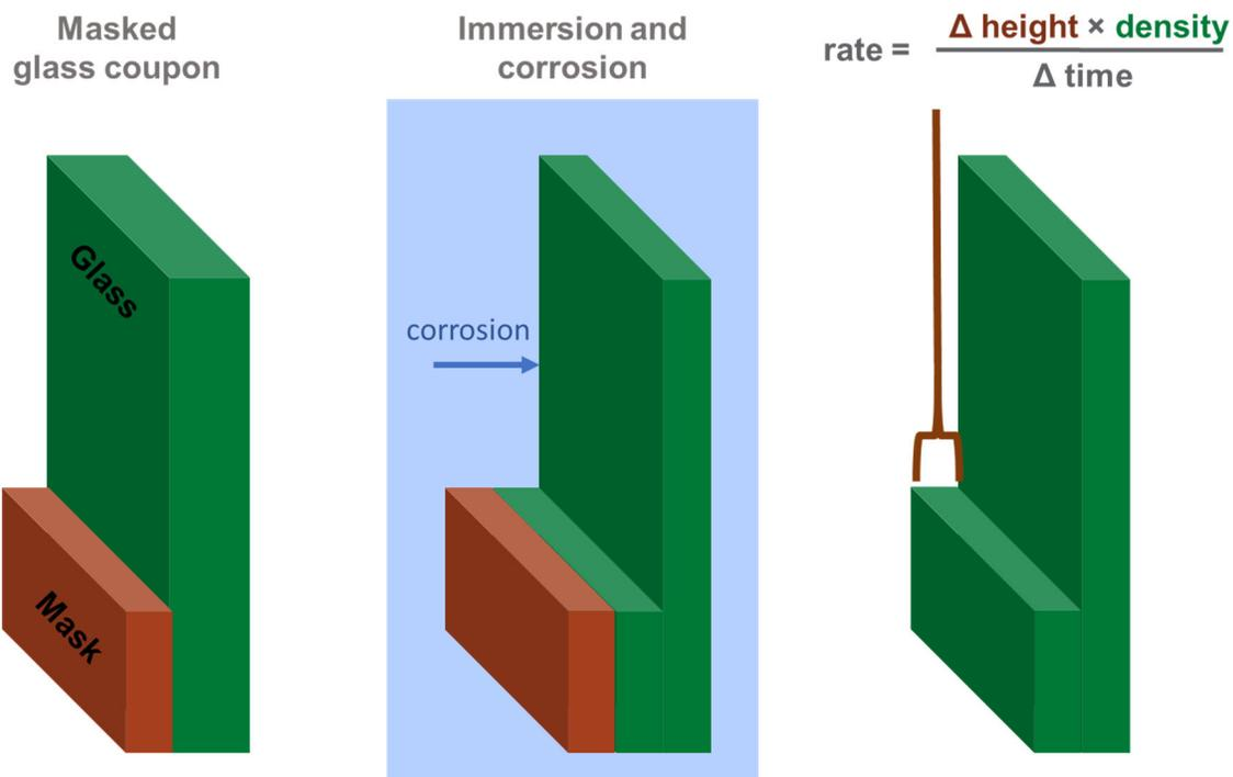
Figure 1-1. Schematic of glass coupon SRCA technique before corrosion (left), during corrosion (center), and during characterization (right).
