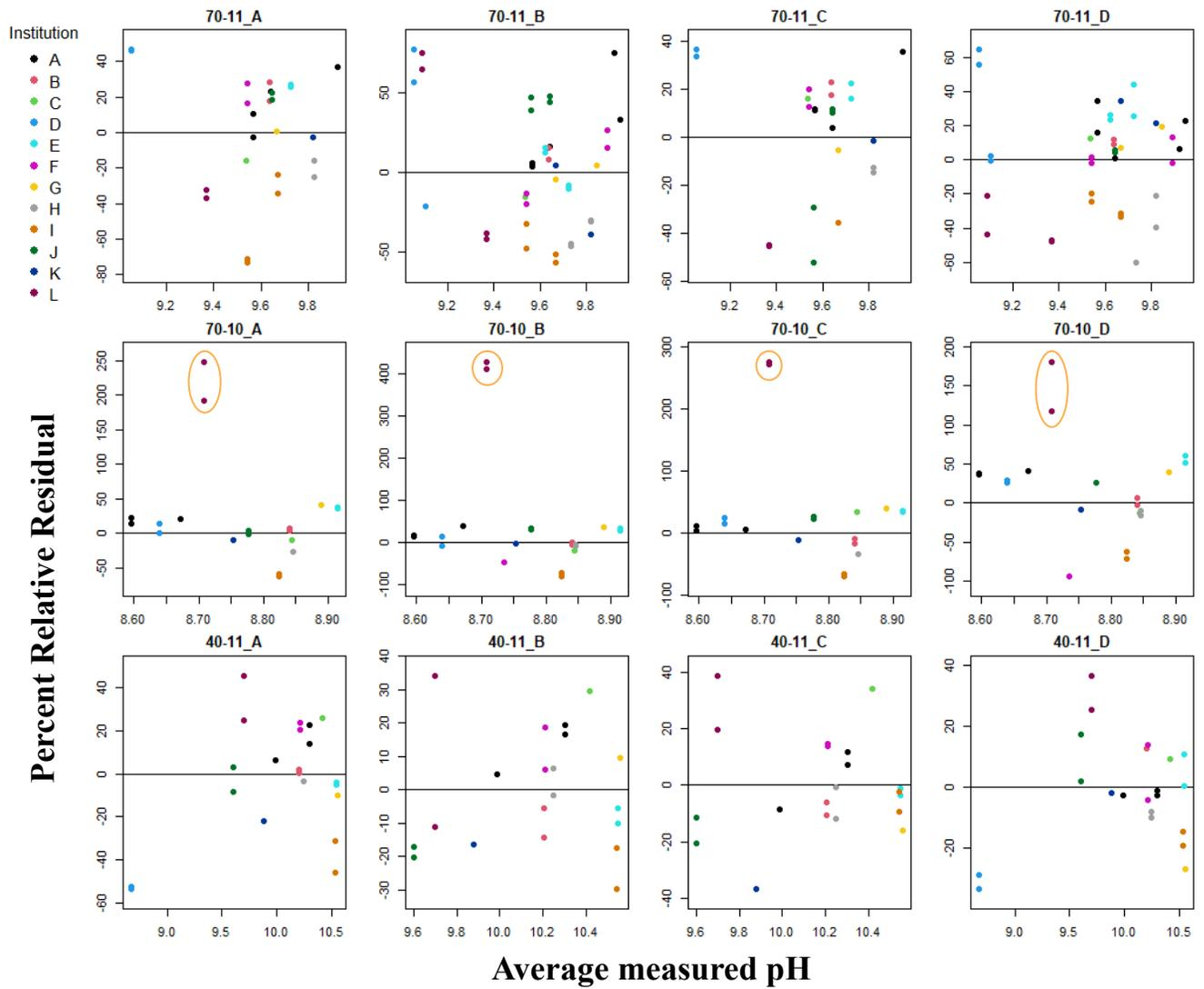
Figure 4-3 - Plot of the departure in % of value from the best linear fit of pH dependence in the given condition as a function of pH. Outlier data points from the  $pH_{(RT)} = 10$  and  $70^\circ\text{C}$  conditions that were excluded from further analysis are circled in orange.
