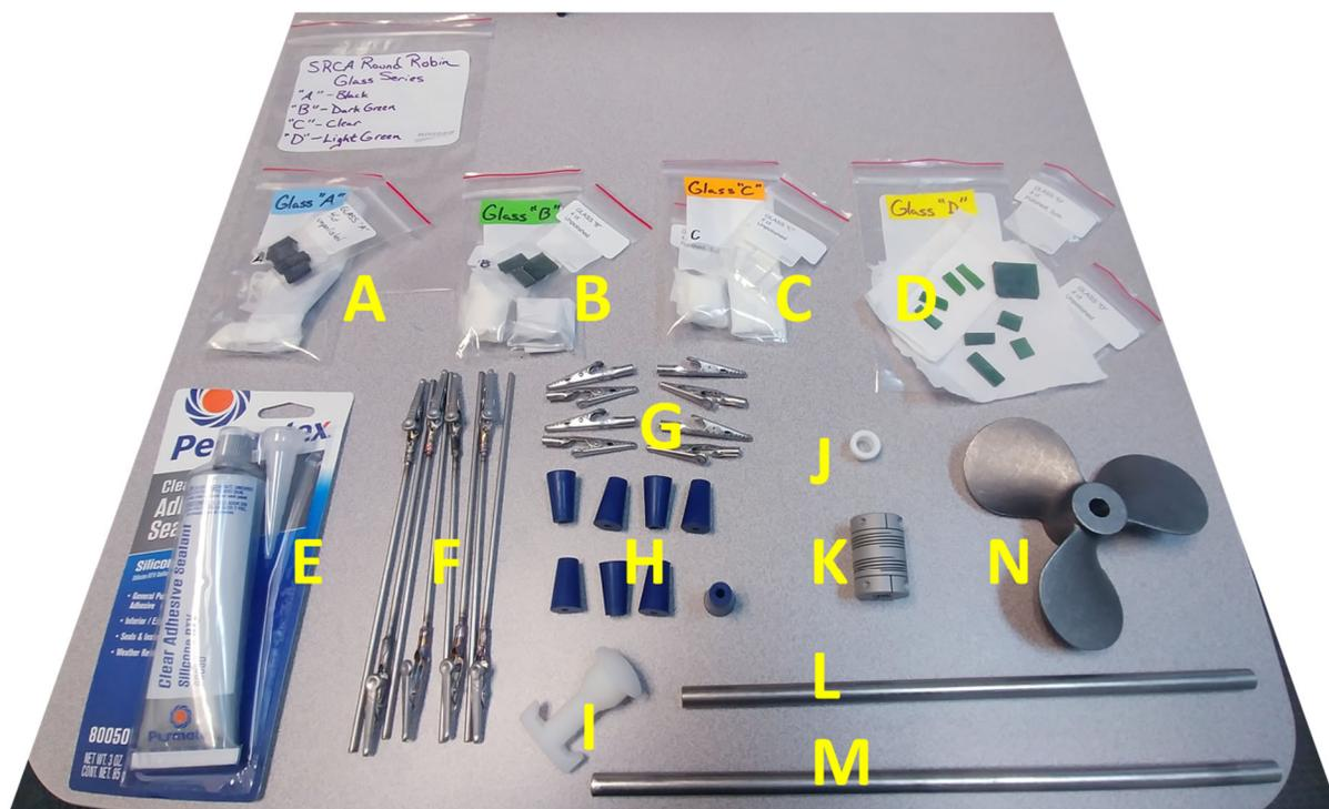
Figure 2-2 - Image of SRCA test apparatus component items shipped to collaborators to complete round robin testing. 10" diameter × 10" deep stainless-steel vessel and lid not shown.
