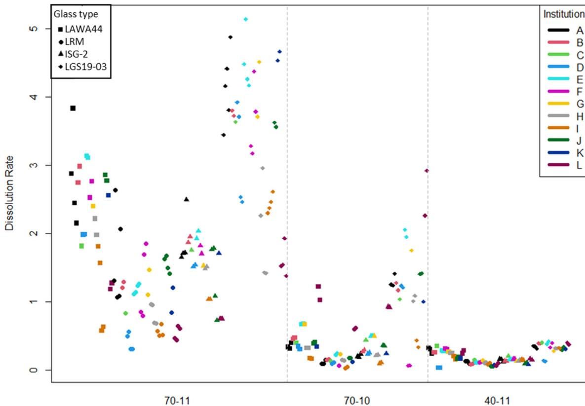
Figure 3-1 - Dilute dissolution rates ( $\text{g}\cdot\text{m}^{-2}\cdot\text{d}^{-1}$ ) for all tests completed as part of the round robin test matrix. Nominal conditions are called out in the X-axis.
