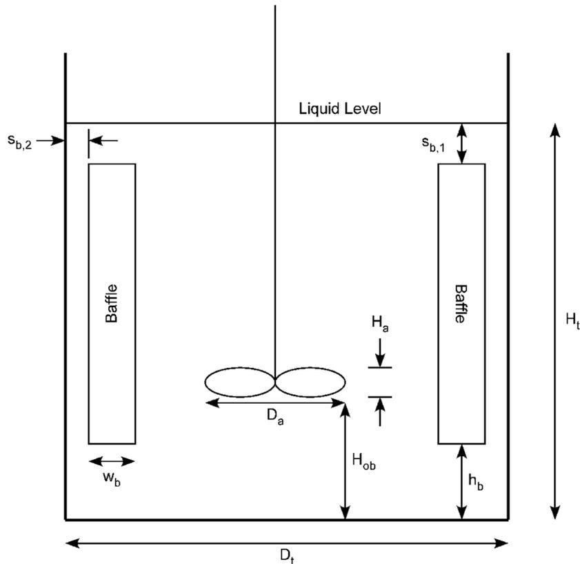
Figure 6-3. General schematic of baffled flat-bottom reactor with important dimensions.
