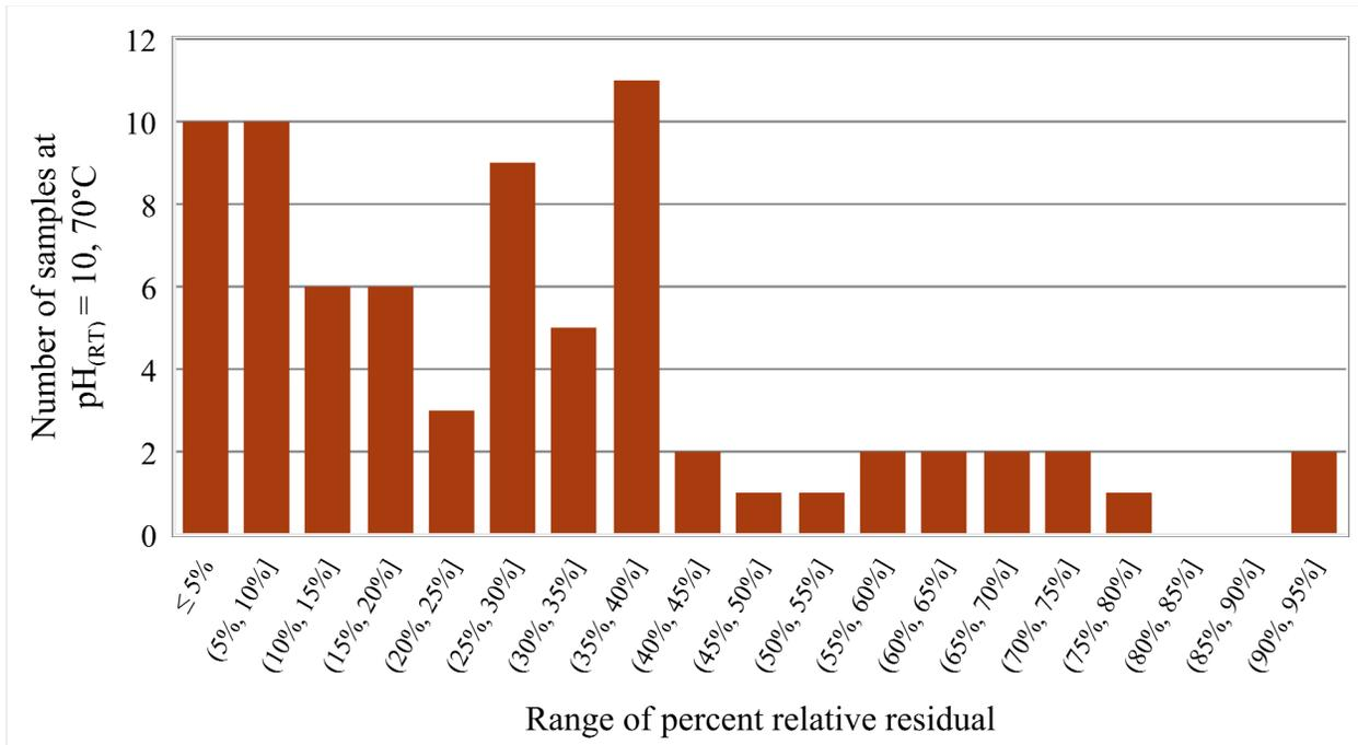
Figure 4-6 – The distribution of percent relative residual values for all samples tested at  $pH_{(RT)} = 10, 70\text{ }^{\circ}\text{C}$
