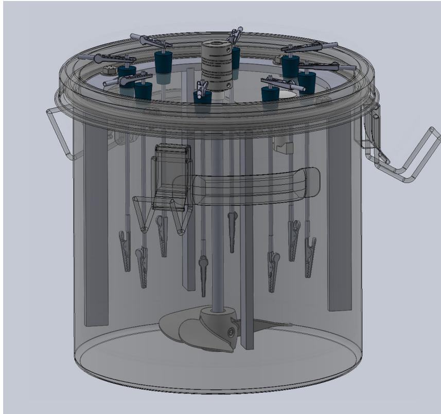
Figure 6-1 - Schematic of a the dilute reactor SRCA design used for the precision round robin studies
