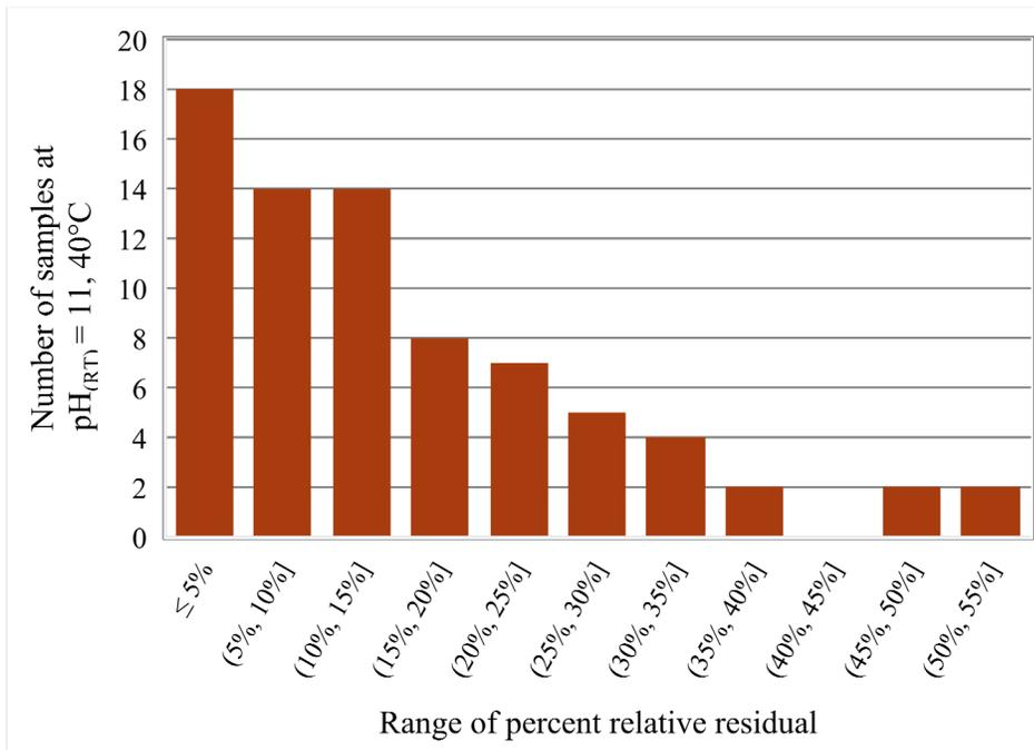
Figure 4-7 – The distribution of percent relative residual values for all samples tested at  $pH_{(RT)} = 11, 40\text{ }^{\circ}\text{C}$
