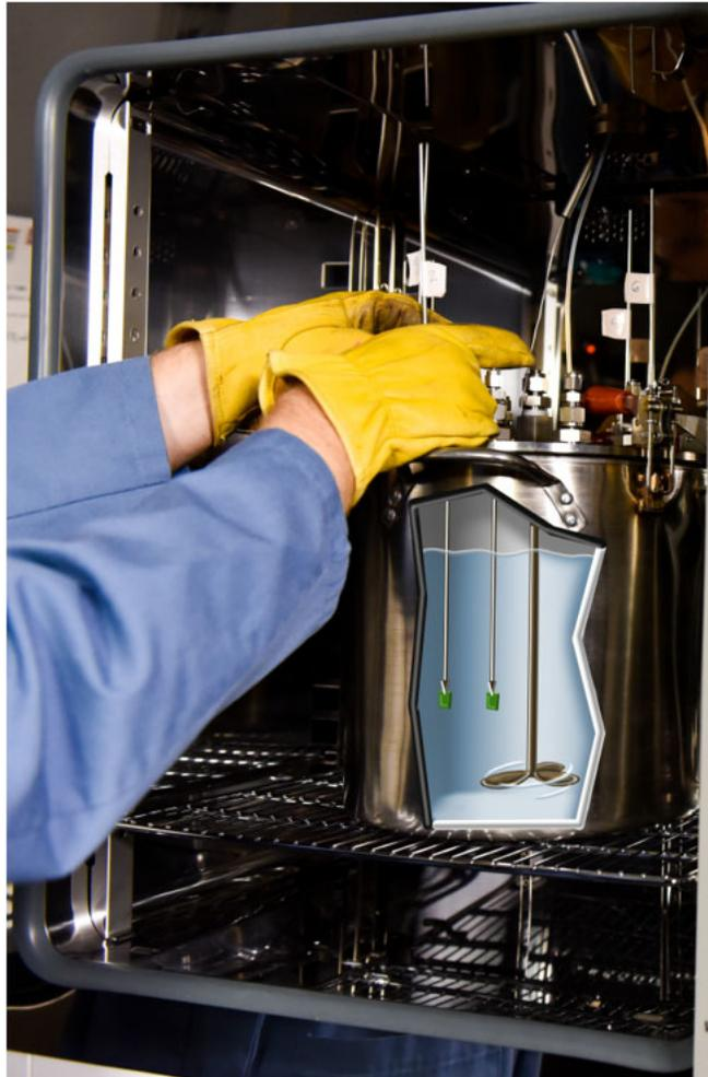
Figure 2-1. A photograph with cutaway schematic of the SRCA design for a large (11 L) stainless steel reactor.
