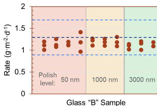
Figure 6-2 - Single vessel replicates of Glass "B" showing repeatability and no impact of polish quality on results.
