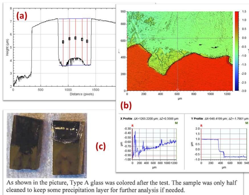
Figure 3-2 – Evidence of alteration layers from three collaborators following tests at  $\text{pH}_{(\text{RT})}=11$  and  $70^\circ\text{C}$  on (a) LGS19-03 glass (stylus profilometry), (b) LGS19-03 glass (optical profilometry), and (c) LAWA44 glass (optical picture and notes)
