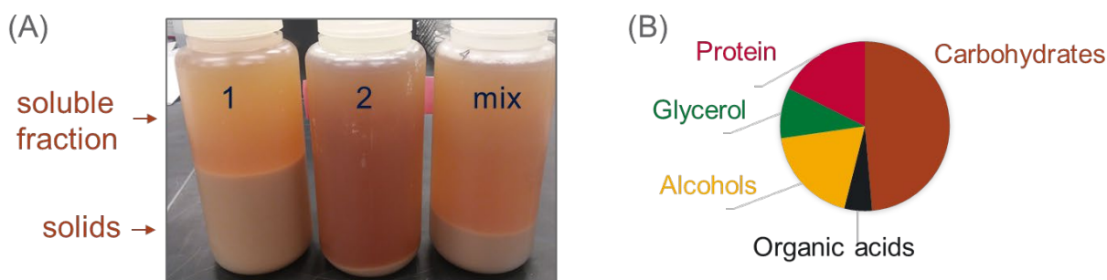
Figure 1. Stillage samples from Solar Spirits (Richland, WA). (A) Stillage samples from distillation 1 and 2 after centrifugation. (B) Compositional makeup of the soluble fraction from a mixture of distillation 1 and 2 used for experimental work.
