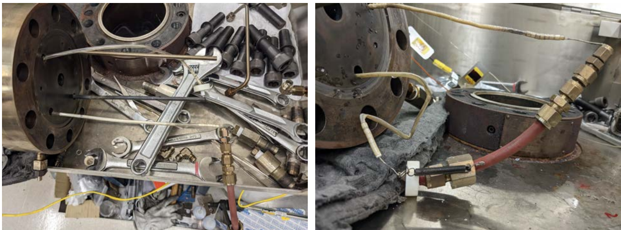
Figure 75: PNNL Fixture Design #3 (before and after 288°C testing inside an autoclave with PWR water)
