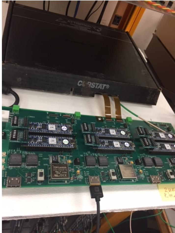
Figure 21. The improved detector in a box and connected to an FPGA board.
