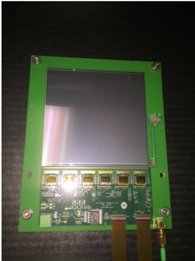
Figure 20. New PCB with silicon strip detector and bonded ASIC.
