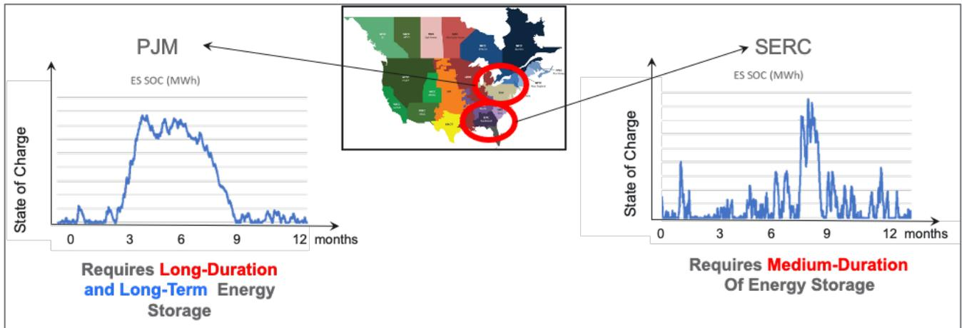
Figure 1: Optimal State of Charge over a Period of 1-year for two Regions
