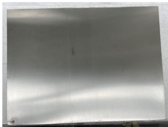
Figure 12. The Zr sheet following wet polishing at 3M.
