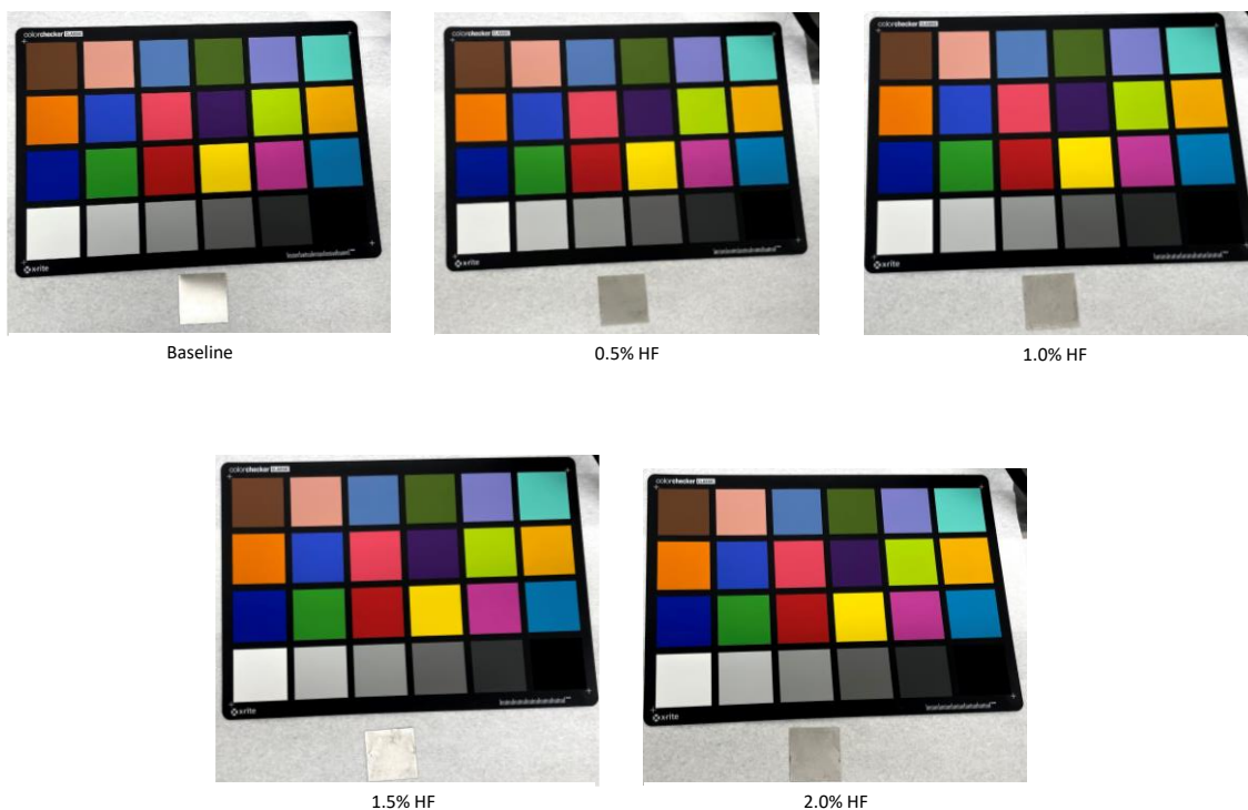
Figure 17. Flash etching Set 1 samples compared to a color chart. Each etched sample had brown staining and more of a matte finish than the shinier, silver baseline sample.
