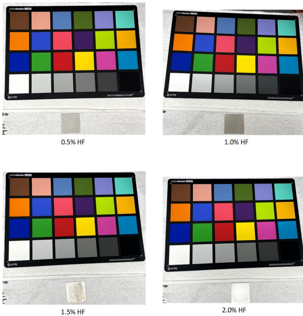
Figure 23. Set 3 samples etched at 30 wt% nitric and varying hydrofluoric concentrations compared to a color chart. Etch time was for 40 seconds.
