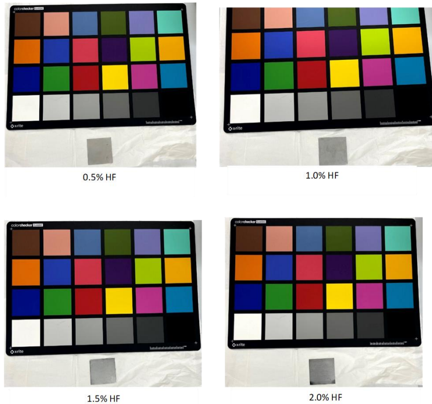
Figure 29. Comparison of the Set 5 post-etch samples and a color chart etched in 40wt% HNO 3 at varying HF concentrations. Etch time was 40 seconds.
