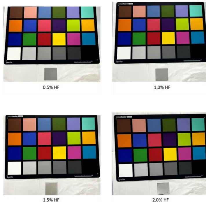
Figure 26. Comparison of the Set 4 post-etch samples and a color chart etched in 40wt% HNO 3 at varying HF concentrations. The etch time was 20 seconds.
