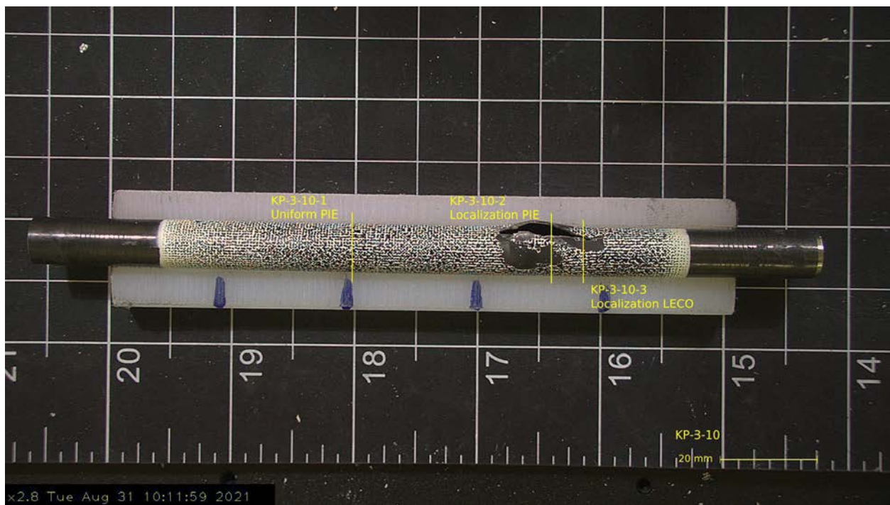
Figure 4-14. Post-Burst Image of KP-3-10 (Room Temperature / Higher Burnup)
