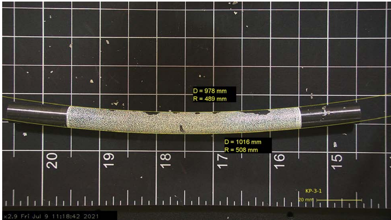
Figure G-44. Post-Bend Image of KP-3-1 with Radius of Curvature Measurement
