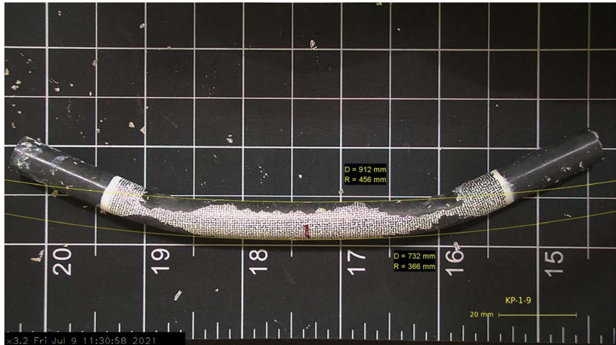
Figure G-33. Post-Bend Image of KP-1-9 with Radius of Curvature Measurement
