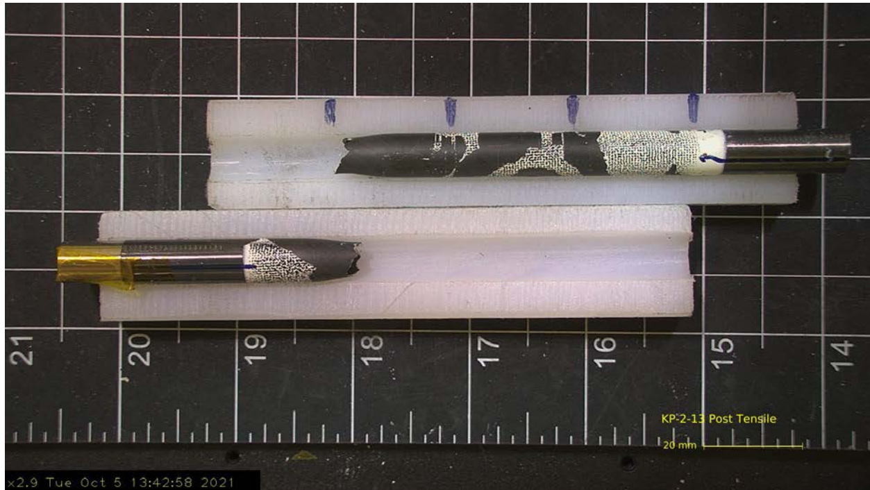
Figure 3-27. Post-Tensile Sample KP-2-13 (Room Temperature / Grid Spacer)
