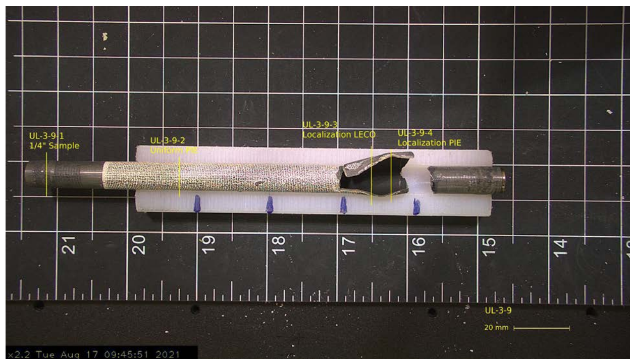
Figure 4-9. Post-Burst Sample UL-3-9 (200°C / Higher Burnup)
