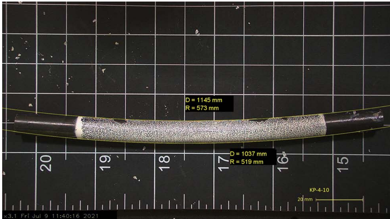
Figure G-55. Post-Bend Image of KP-4-10 with Radius of Curvature Measurement
