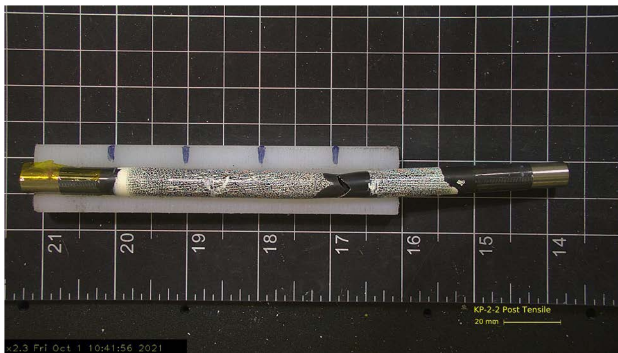
Figure 3-26. Post-Tensile Sample KP-2-2 (Room Temperature / Higher Burnup)
