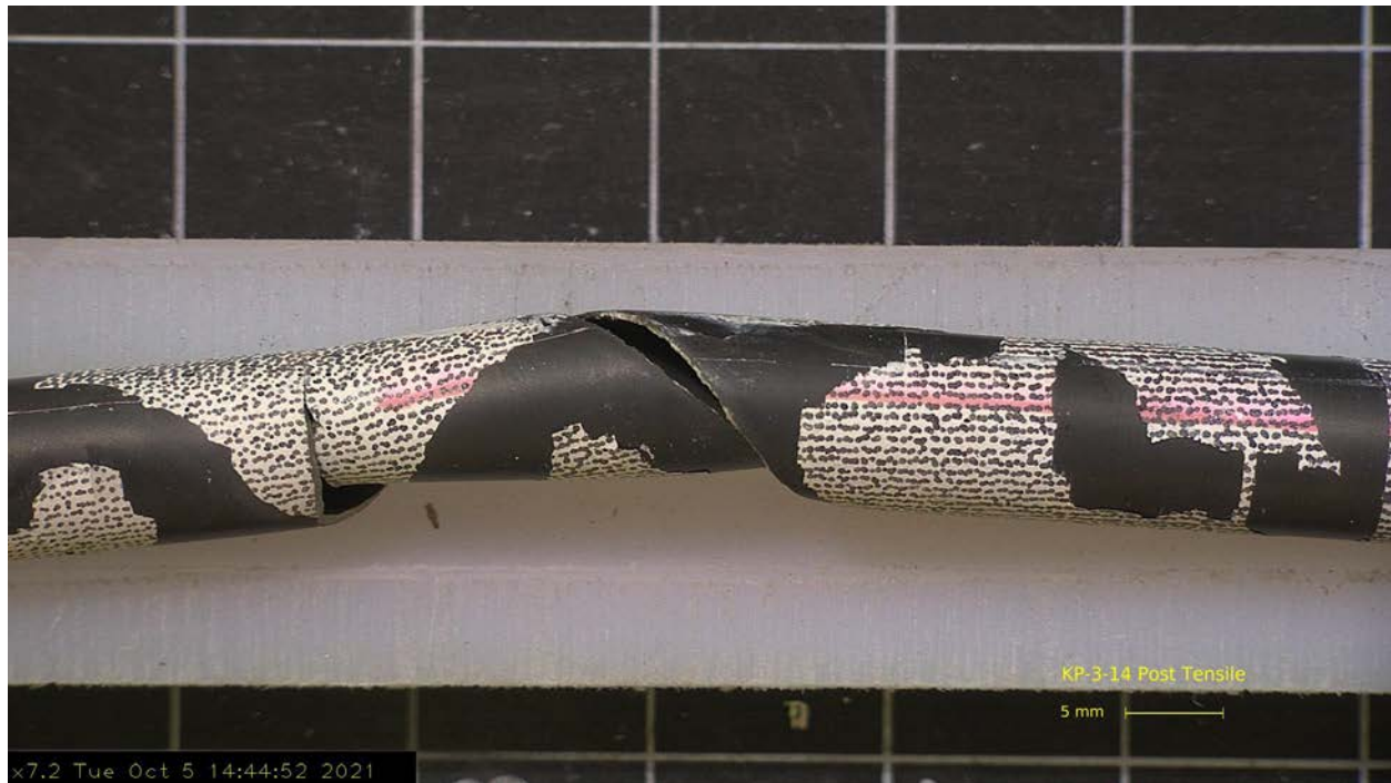
Figure E-211. Post-Tensile Image Side 1 of Fracture for KP-3-14
