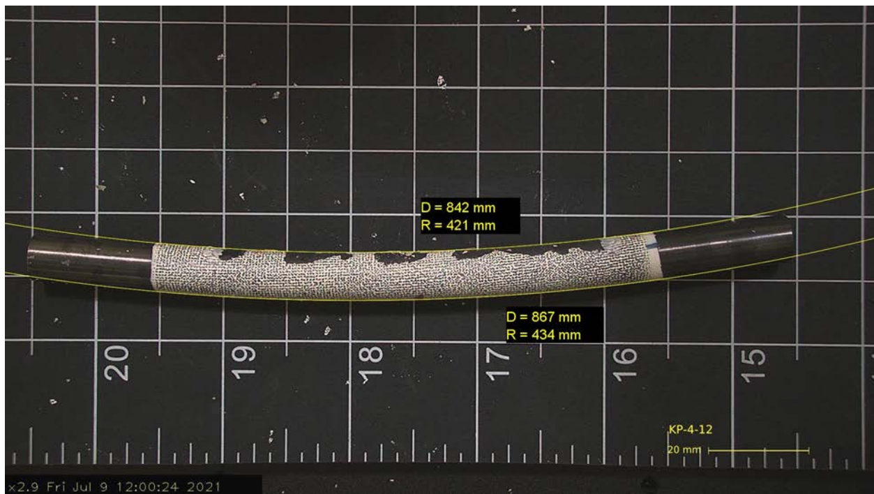
Figure 5-18. Post-Bend Radius of Curvature Measurement of KP-4-12
