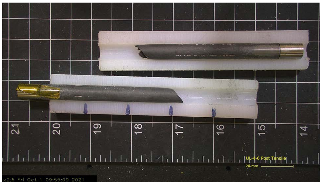
Figure 3-11. Post-Tensile Sample UL-4-6 (Room Temperature / Lower Burnup)
