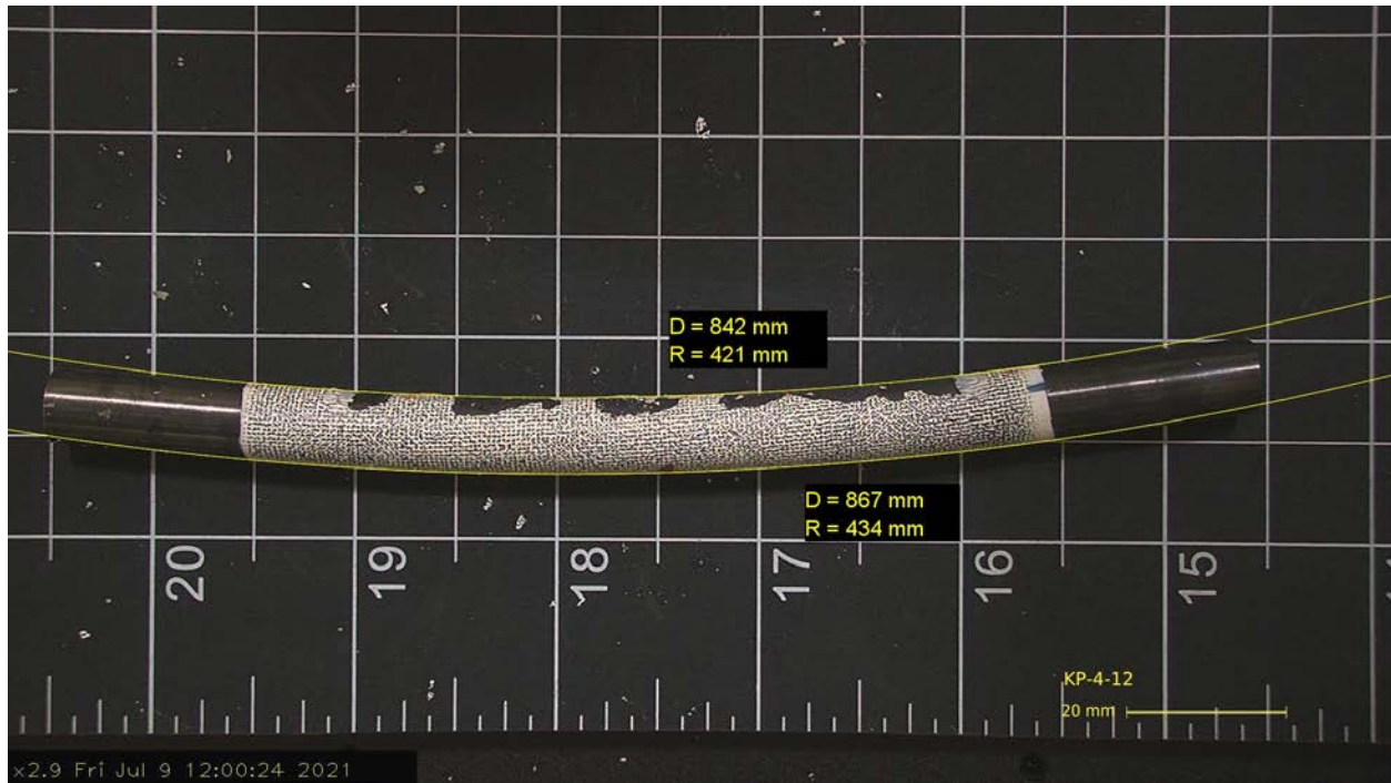
Figure G-66. Post-Bend Image of KP-4-12 with Radius of Curvature Measurement
