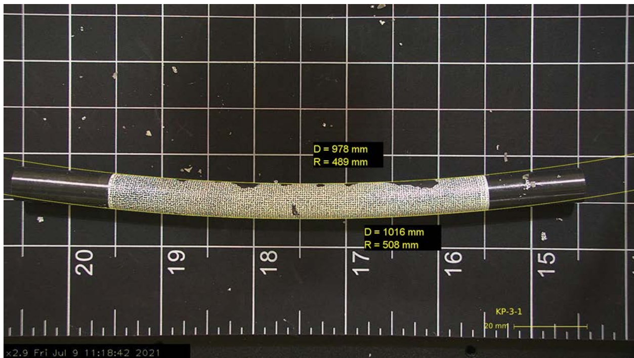
Figure 5-16. Post-Bend Radius of Curvature Measurement of KP-3-1
