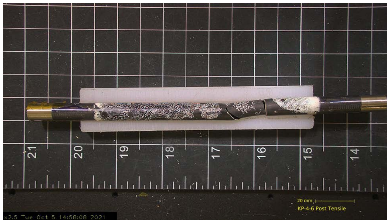
Figure 3-25. Post-Tensile Sample KP-4-6 (Room Temperature / Lower Burnup)
