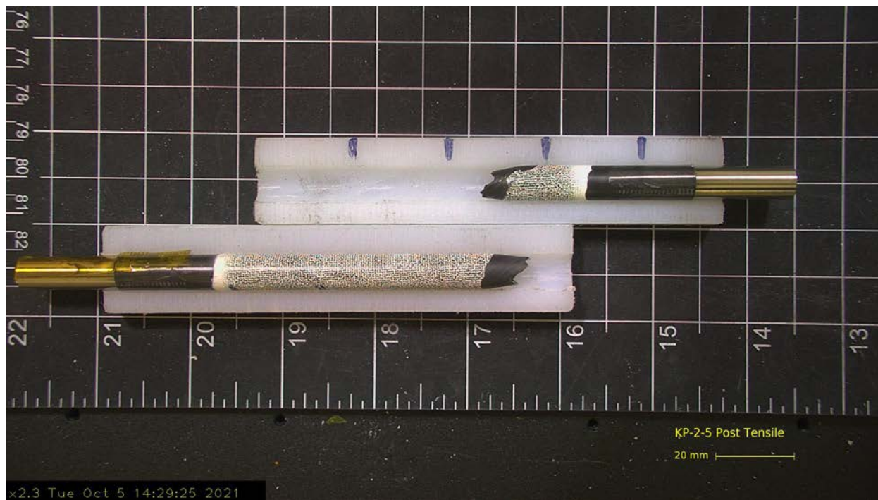
Figure 3-30. Post-Tensile Sample KP-2-5 (200 °C / Grid Spacer)
