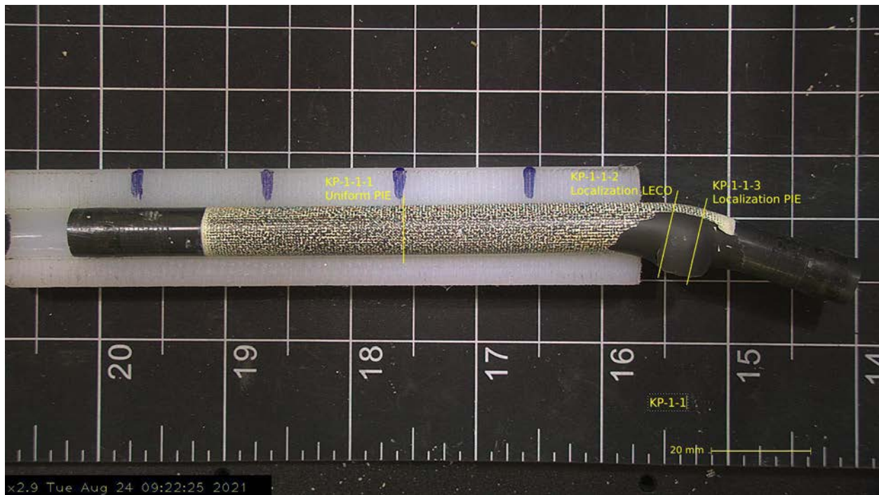
Figure 4-17. Post-Burst Image of KP-1-1 (200°C / Lower Burnup)
