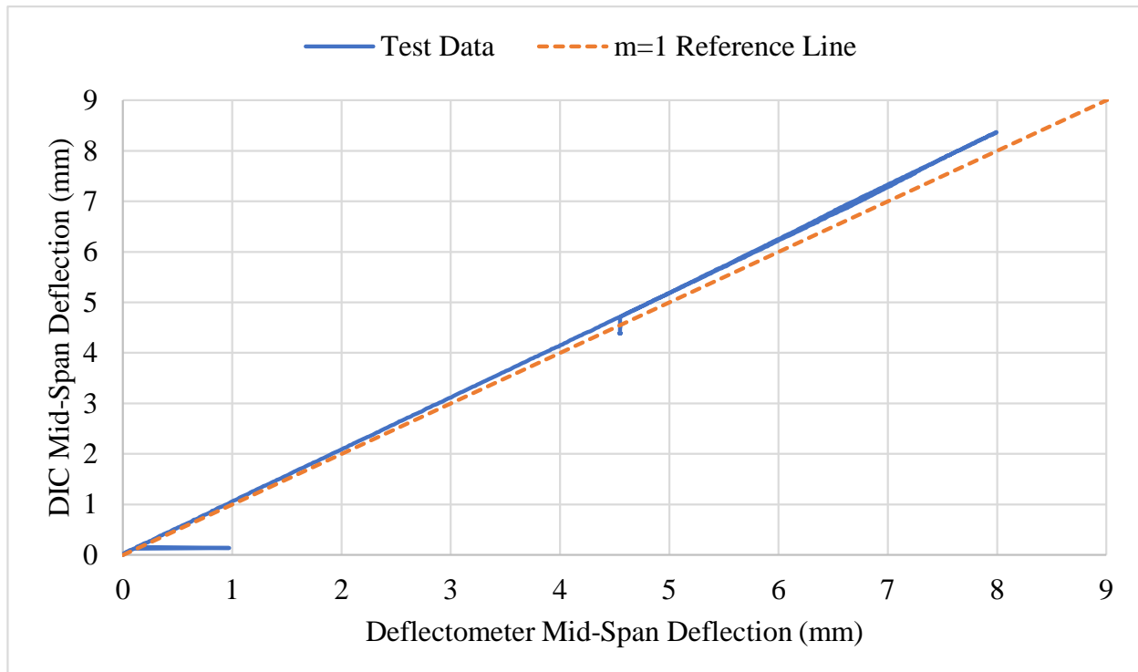
Figure G-71. Comparison of Bluehill and DIC Mid-Span Deflection for KP-4-2
