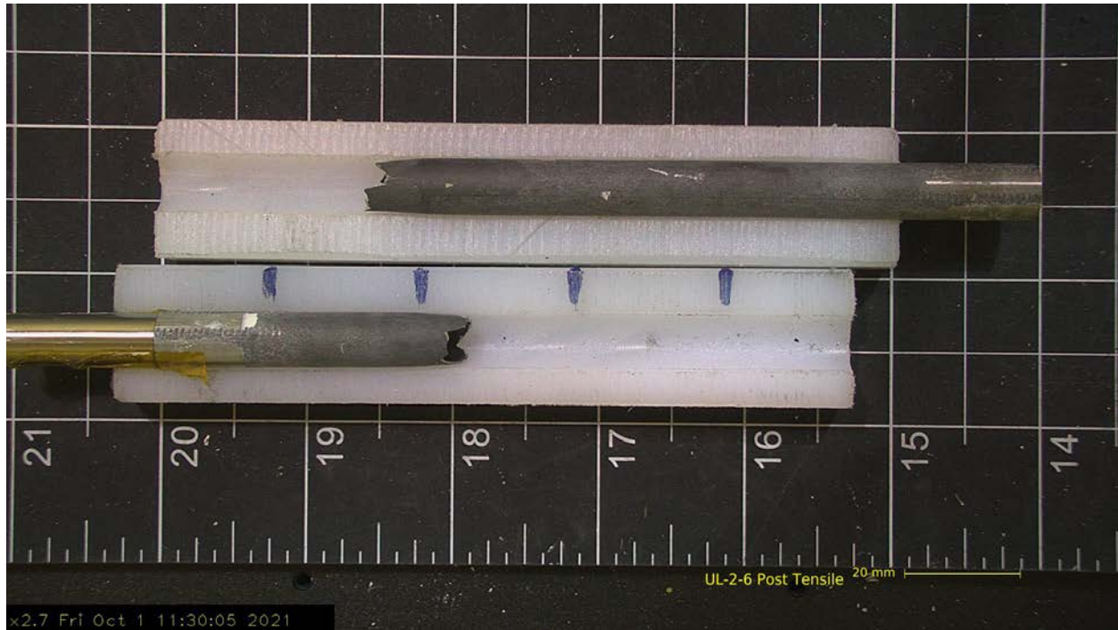
Figure 3-17. Post-Tensile Sample UL-2-6 (200°C / Grid Spacer)
