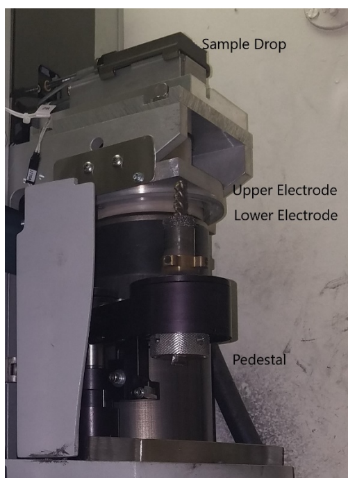
Figure B-2. Lower Electrode Raised to Meet the Upper Electrode
