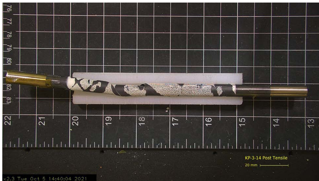
Figure 3-29. Post-Tensile Sample KP-3-14 (200°C / Higher Burnup)
