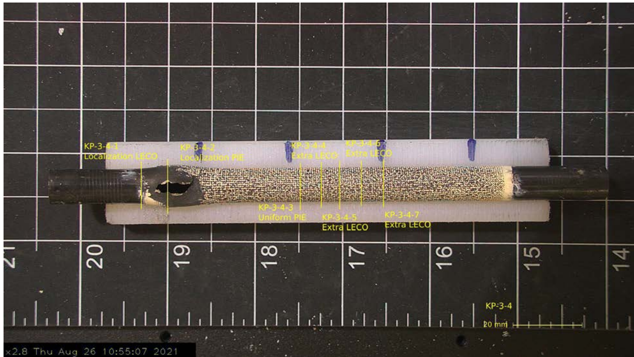
Figure 4-15. Post-Burst Image of KP-3-4 (200°C / Higher Burnup)
