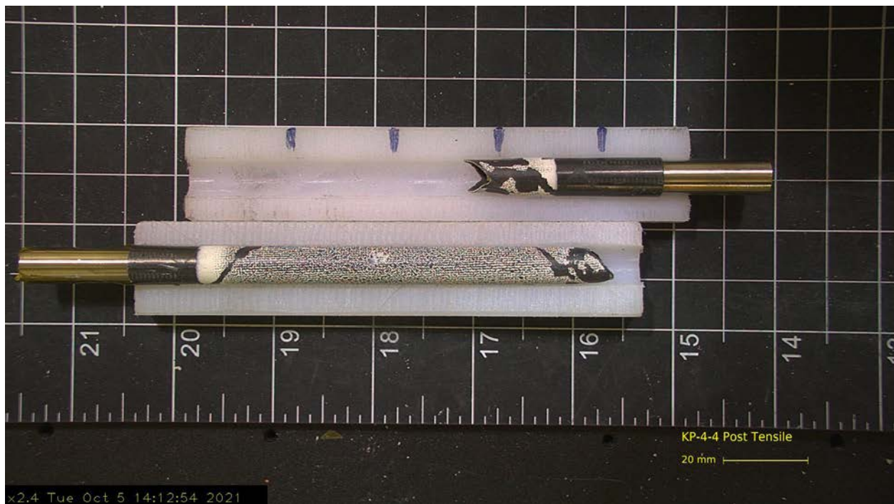
Figure 3-28. Post-Tensile Sample KP-4-4 (200°C / Lower Burnup)
