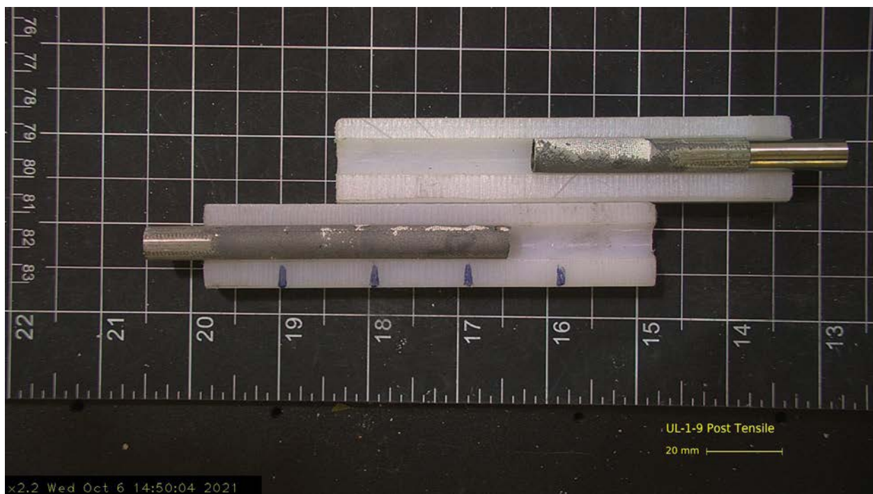
Figure 3-14. Post-Tensile Sample UL-1-9 (Room Temperature / Lower Burnup / High Hydrogen)
