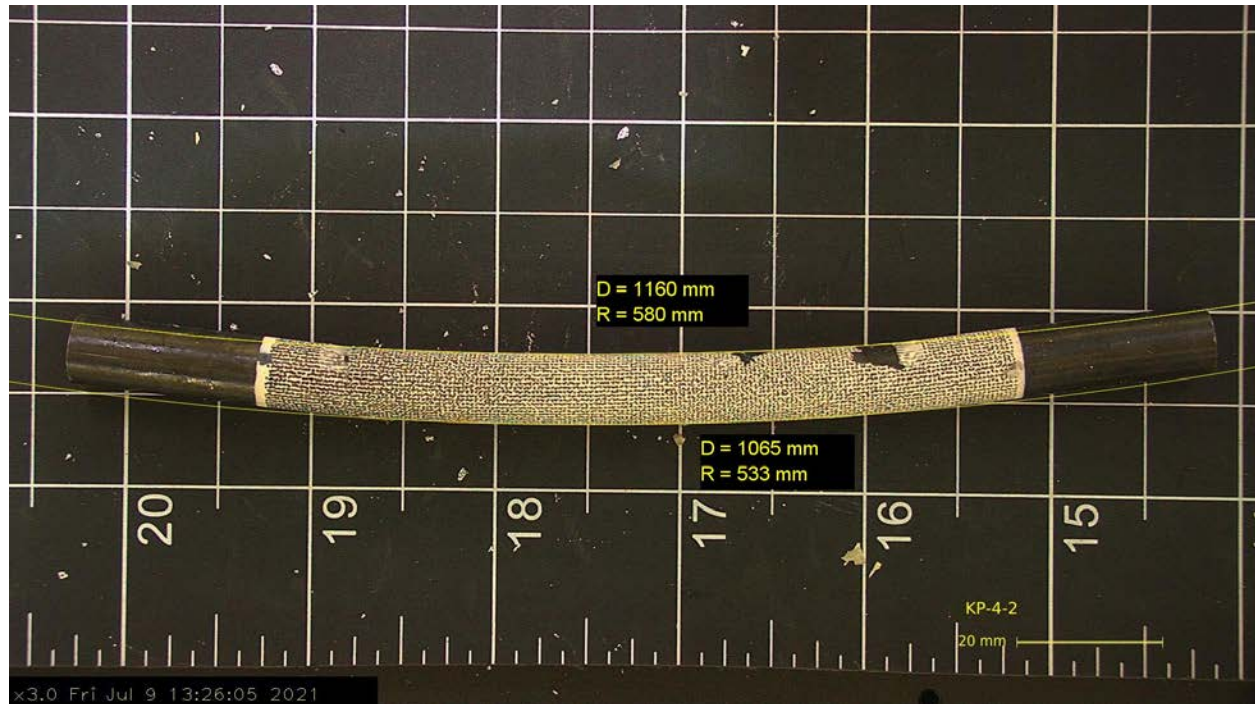
Figure G-77. Post-Bend Image of KP-4-2 with Radius of Curvature Measurement
