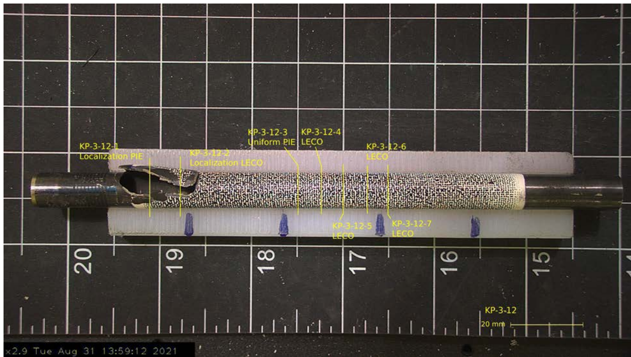
Figure 4-13. Post-Burst Image of KP-3-12 (Room Temperature / Grid Spacer)
