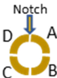
Figure 2-2. Quadrant Identification for Total Hydrogen Analysis
