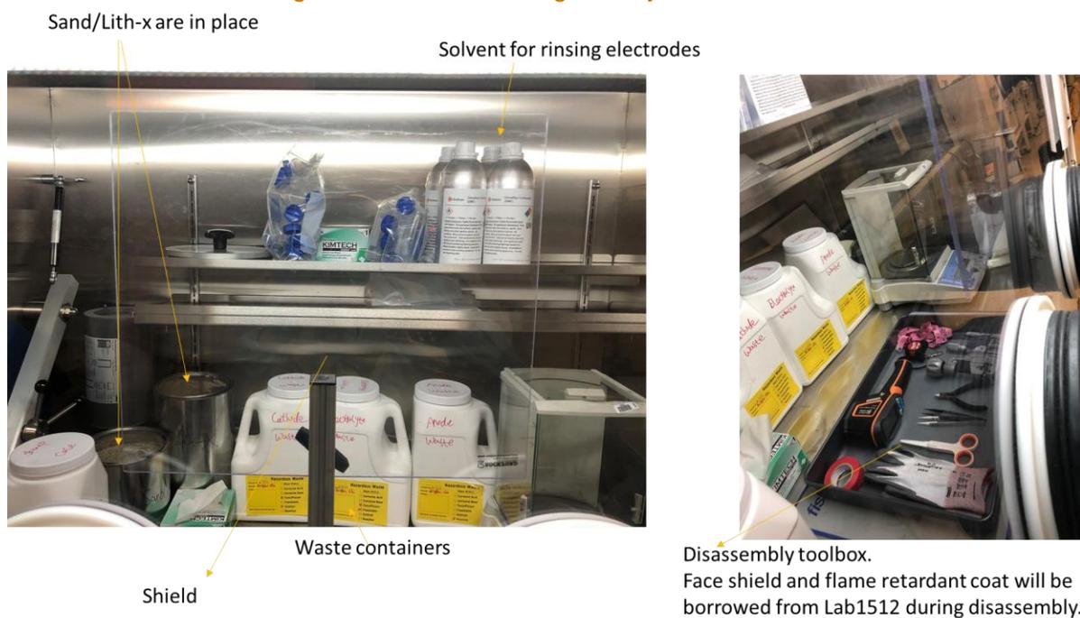
Fig.24 Setup for cell disassembly of commercial 18650/21700 LIBs at PSL 522A.
