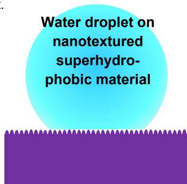
**Water droplet on nanotextured superhydrophobic material**
