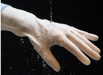
The flexible coating can be easily applied to PPE surfaces making water bead and shed smoothly.
