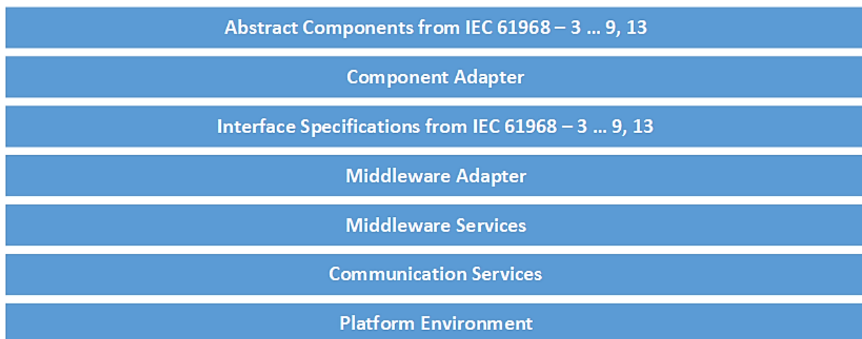
Figure 11: Interface layers defined in the IEC 61968-1 Standard [21]
