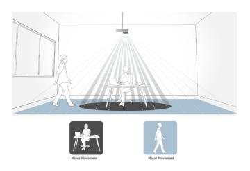
The timeout period represents the length of time the sensor must detect a stable response (no motion) before signaling lights to turn off. If the sensor detects motion within the timeout period, lights stay on and the timeout period resets.
