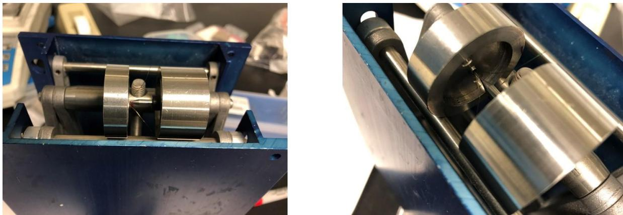
Fig.11 Home-made alignment tools (includes a lift table or lab jack, top and bottom crimping die) for drilling a hole at the center of the cathode.
