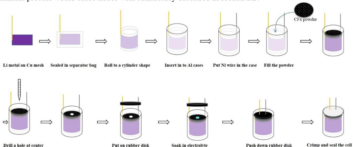
Fig.5 Schematic of a typical procedure for producing Gen2 micro battery (MB1842).
