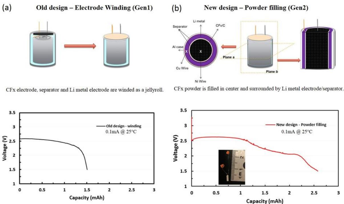
Fig.2 Cell structure and cell performance of Lamprey micro batteries (MB1842) with a) old design (Gen1) and b) new design (Gen2).
