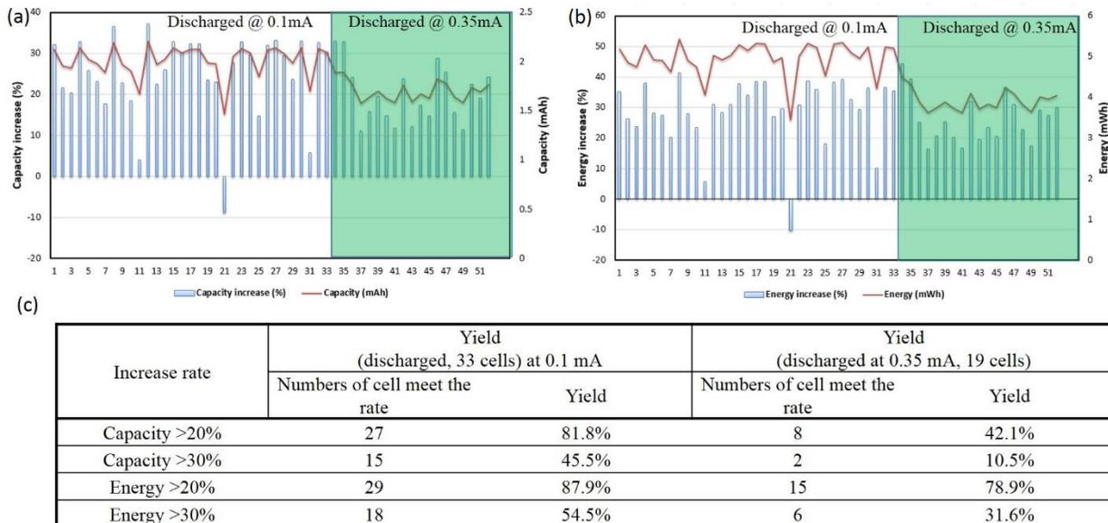
Fig.9 a) Capacity increase, b) energy increase and c) yield analysis for trial run in Fig.8.
