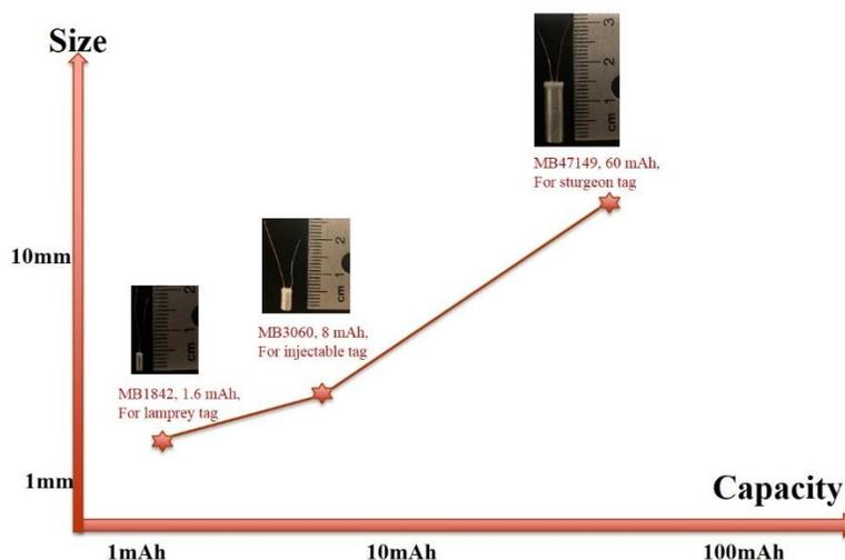
Fig.1 Three types of cylindrical micro batteries (Gen1) developed at PNNL.
