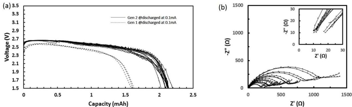
Fig.10 a) Cell performance discharged at 0.1mA and b) Nyquist plot of 15 MB1842 micro batteries with >30% capacity increase rate in Fig.8c.
