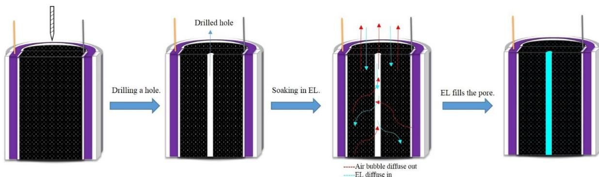
Fig.4 Schematic of proposed second solution to create more pores in Gen2 micro battery.
