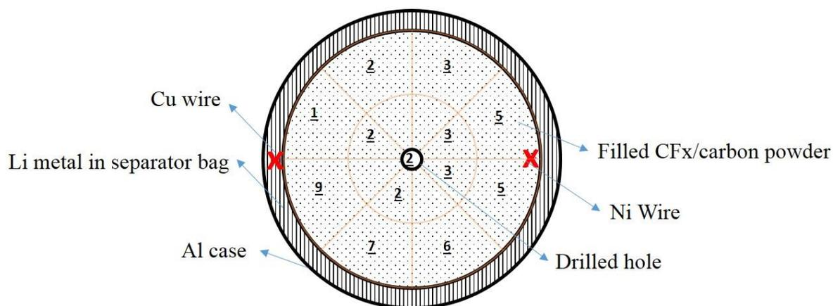
Fig.12 Statistics of the position distribution of the drilled holes in 52 cells during the trial run. Number is the number of cells with drilled hole located in this area.
