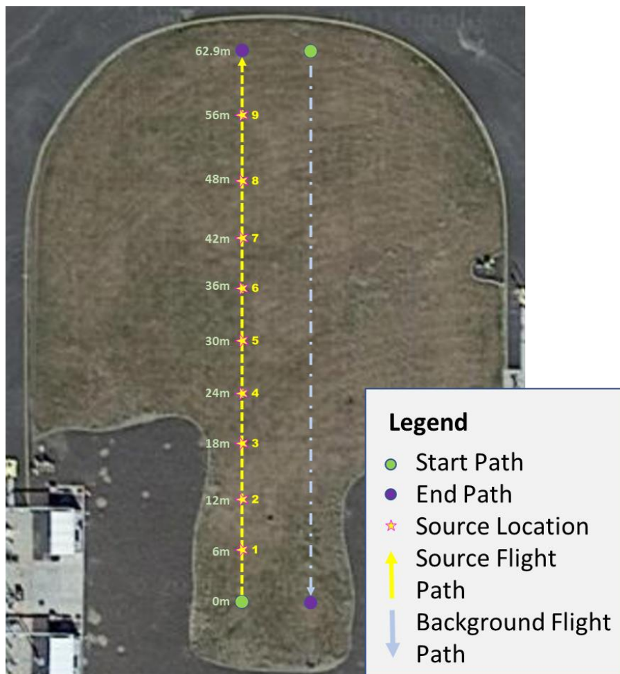
Figure 6. Radiological Survey Field Setup at PNNL's 3440 Test Track
