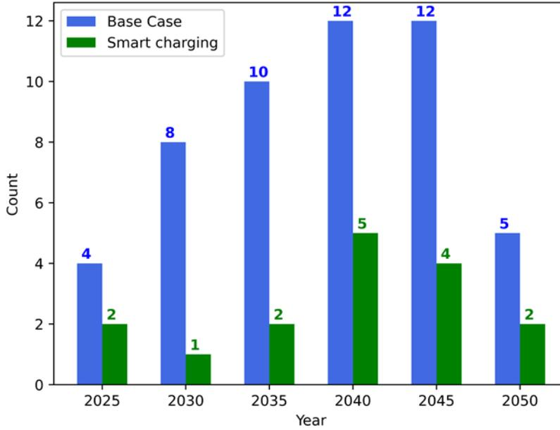
**Figure 17. Transformer upgrade plan for every 5 years with and without SCM**
