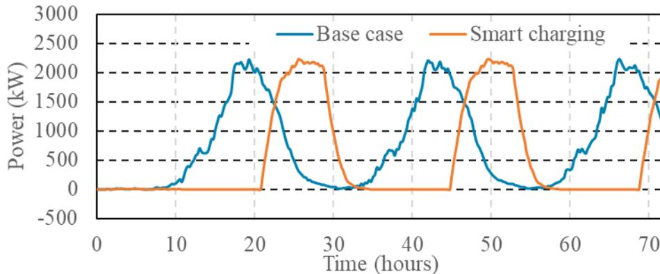
Figure 15. Comparison of the aggregate EV demand profile in base case and smart charging case
