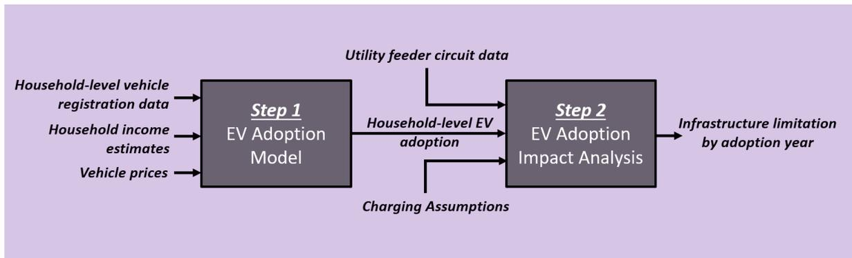
Figure 1. Overall methodology for EV adoption forecast modeling and impact estimation
