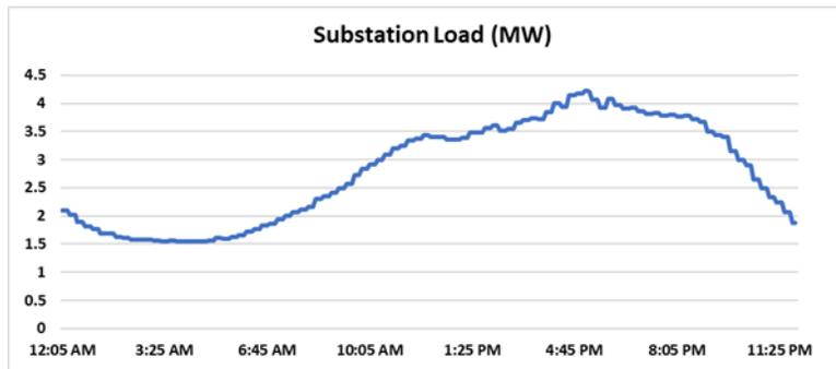
**Figure 4. SCE feeder daily load curve for typical summer weekday with about 176 EVs**
