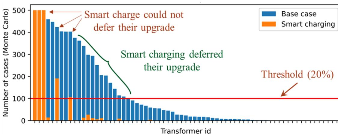
**Figure 16. Monte Carlo cases in which a particular transformer is violated with and without SCM, reflecting SCM's impact on transformer upgrade deferral (results generated for study year 2035)**
