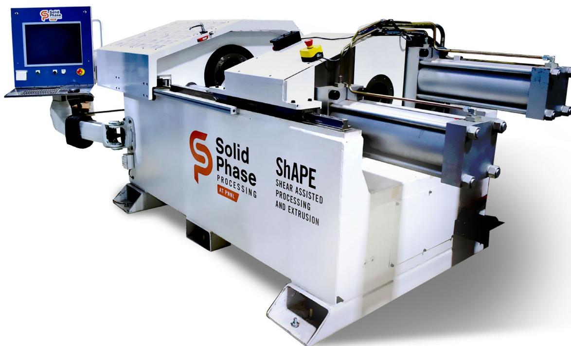
Figure 4. ShAPE Machine manufactured by Bond Technologies, Inc. for PNNL.
