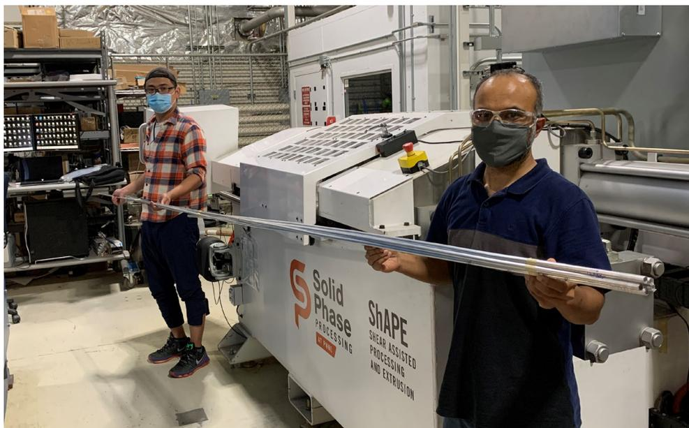
Figure 2. 7075 tubing extruded by ShAPE.
