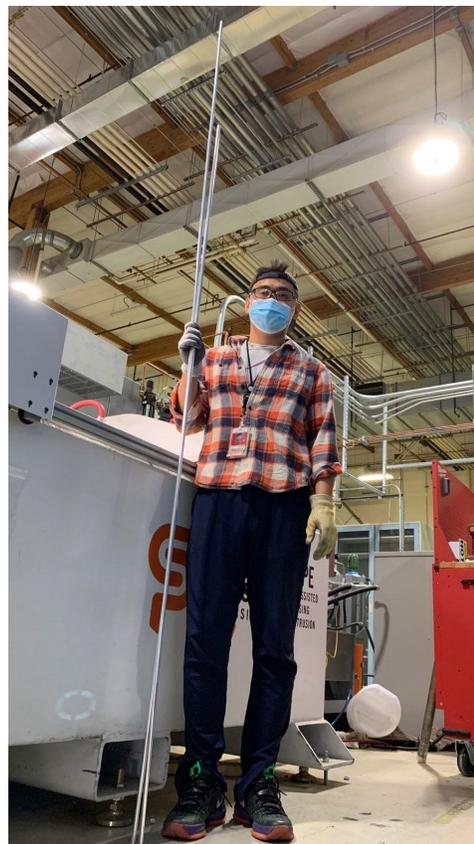
Figure 3. 2024 tubing extruded by ShAPE.
