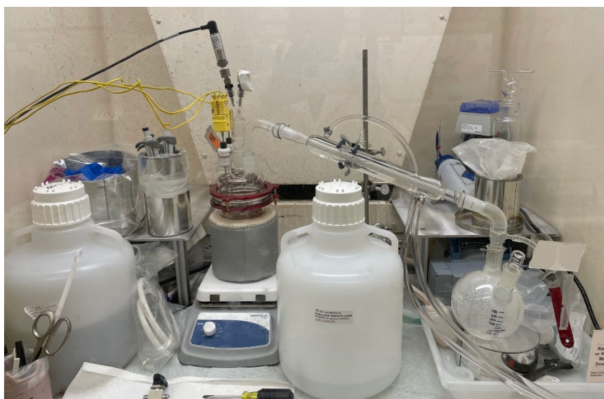
Figure 3.2. EMF evaporator test apparatus as arranged in a CA fume hood.
