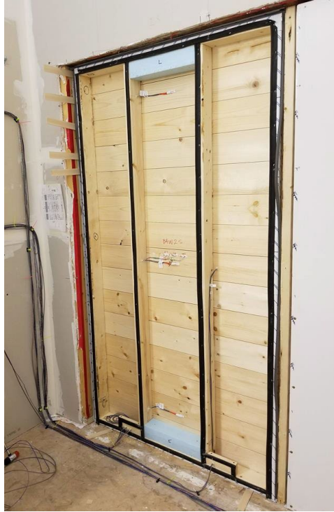
Figure 3-3 All Monitoring Sensors are Within the Center Test Cavity. Wall cavities on each side are guard cavities.
