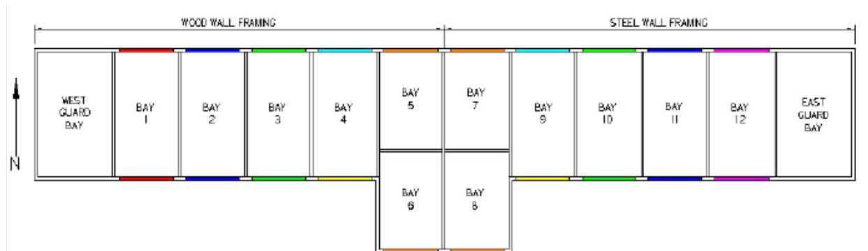
Figure 3-2 Floorplan of the CRRF. Central bays not used; two test walls on each exposure of each bay.
