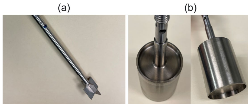
Figure 11. Images of (a) the 16 x 16 mm shear vane tool and (b) Z41Ti viscosity spindle
