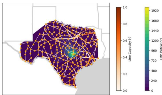
Figure 30. Example of 200-bus real-time LMP and line capacity of their transmission networks during the system peak (2pm August 12, 2016).
