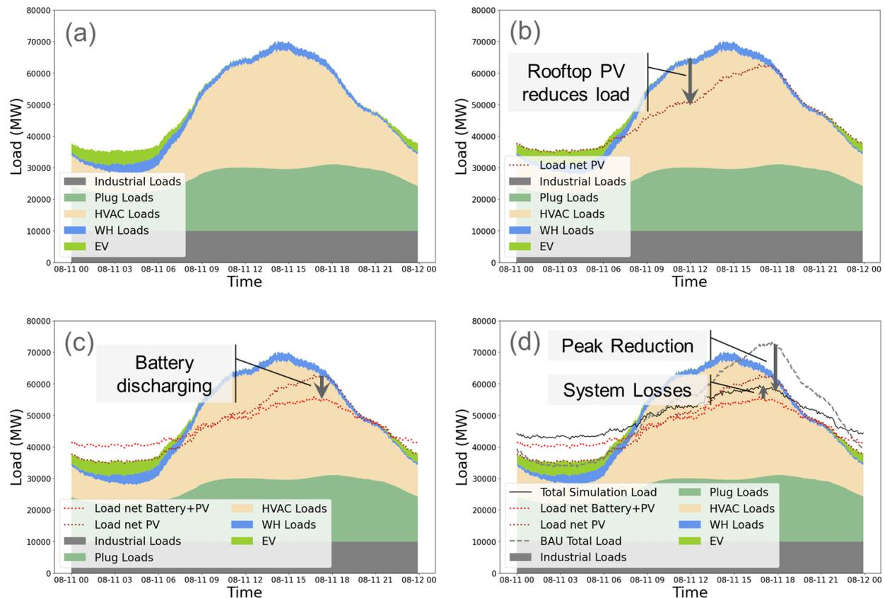
Figure 35. Load profiles plots showing stacked end-use loads (a), the reduction in peak loads due to rooftop solar (b) and battery discharging (c), and the resulting system load (d) after distribution losses are included. (Results shown for the HR battery case.)
