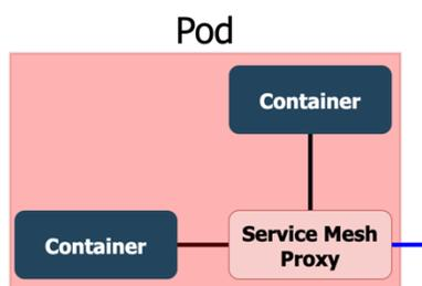
Figure 2. Pods, Containers, and Service Mesh Proxy
