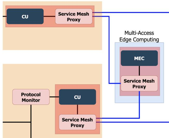
Figure 11. 5G Core Multi-Access Edge Computing (MEC)
