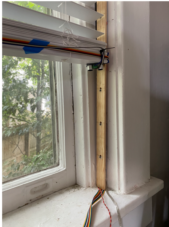
Figure 4.4. Hall effect sensor array tested in this project.
