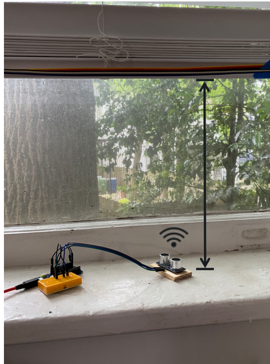
Figure 4.2. An illustrated photo of the sill-mounted ultrasonic distance sensor tested in this project.
