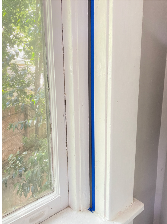
Figure 4.5. The magnetic encoding strip tested in this project.
