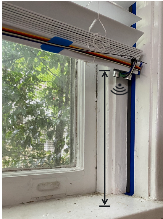
Figure 4.3. Shade-mounted ultrasonic sensor configuration tested in this project.
