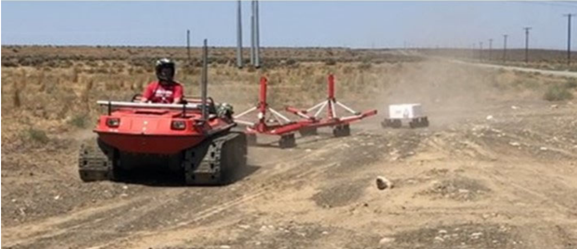
Figure 6. Aarhus tTEM system pulled by an Argo track vehicle.
