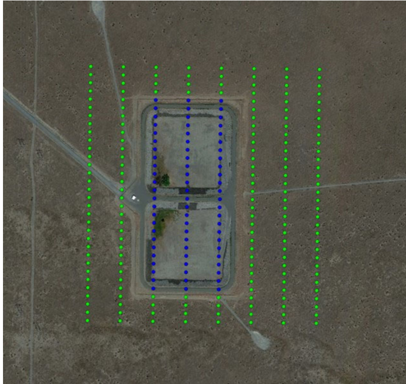
Figure 4. Layout showing which electrodes and cables (i.e. lines) are installed (green) and which are not yet installed (blue).
