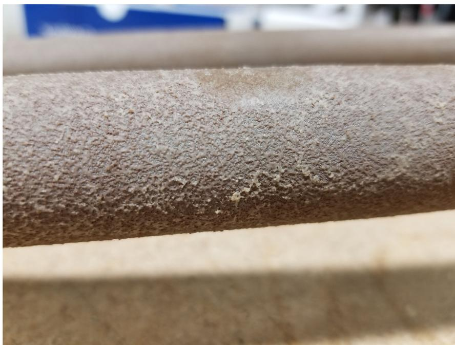
Figure 6.6. Close-Up Image of As-Found Solid Deposits on DEF-01 and DEF-02 Following Test NB1.
