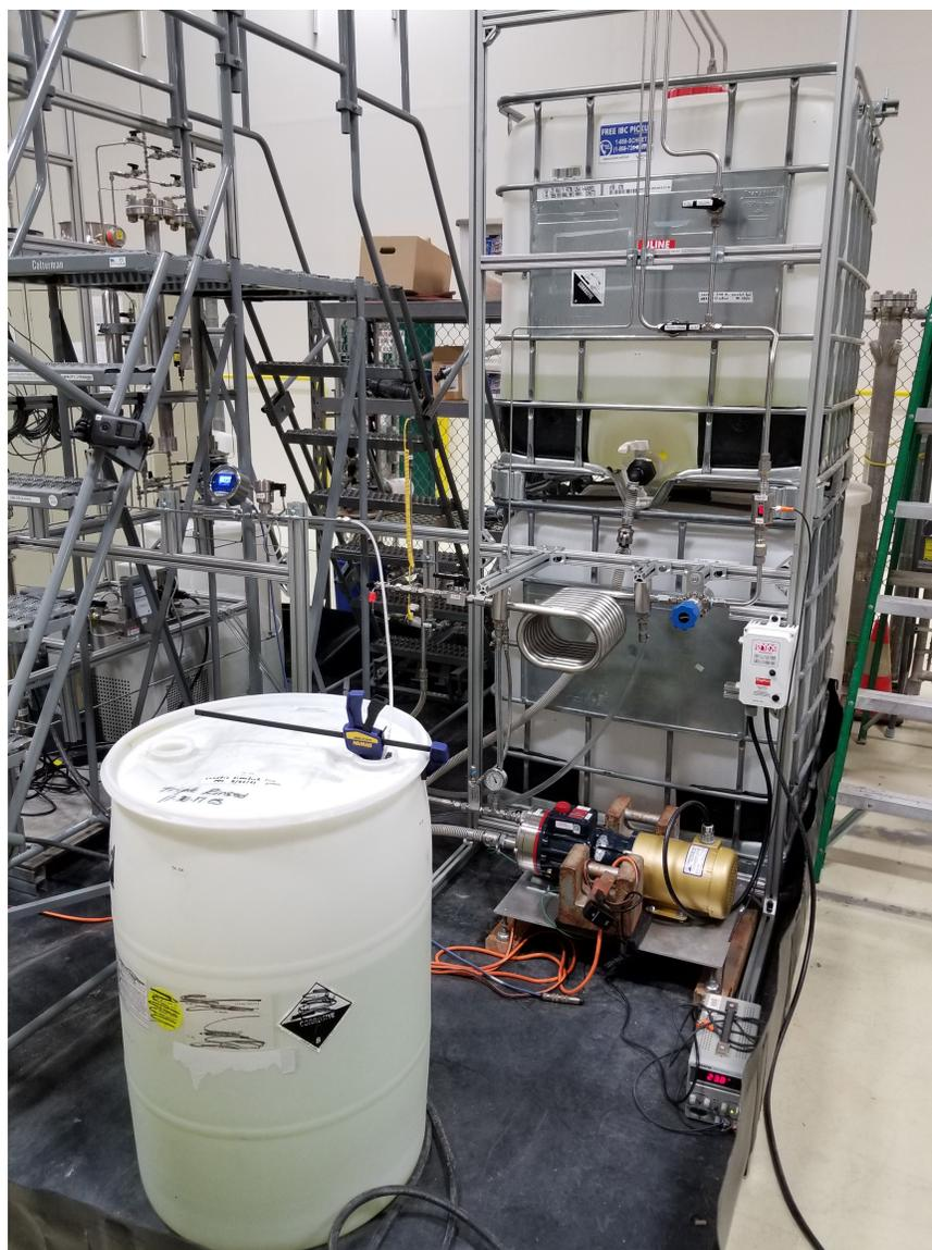
Figure 3.20. Image Showing the Feed Vessel (TK-01) and Recirculation Loop of the Laboratory-Scale High-Solids Test System. On the ground in front of the stacked totes is PMP-01, with TK-01 being the upper tote (partially filled with simulant). The effluent collection vessel TK-04 is in the foreground.
