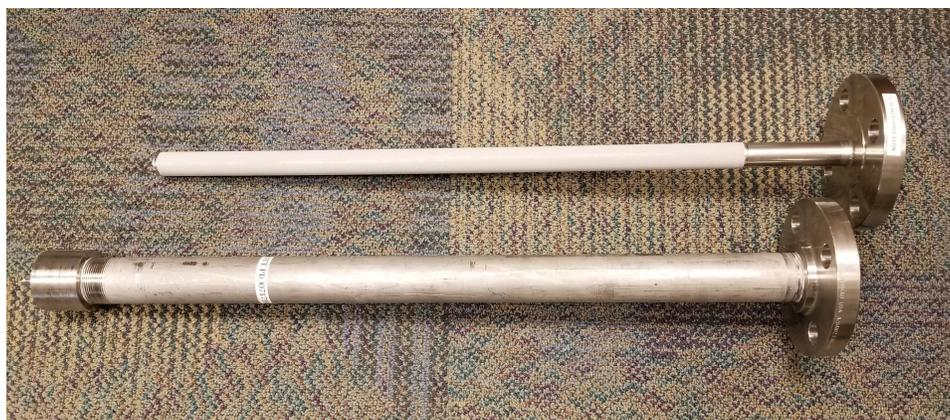
Figure 3.16. Image of Filter Assembly Pieces Side-by-Side before Bolting Together. In the image, the Mott porous element is on the top, and the filter shell is on the bottom.
