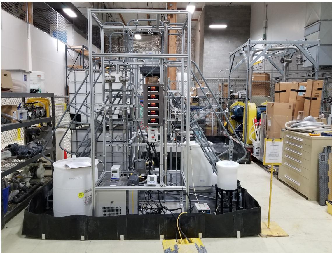
Figure 3.19. Front View of the Laboratory-Scale High-Solids Test System. The DEFs are on the left side of the Bosch frame and the IX column is on the right; outside the frame within the secondary containment is TK-03 (far left) and TK-02 with PMP-02 (far right).
