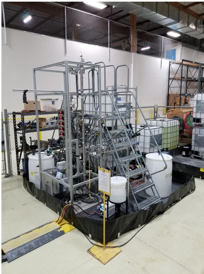
Figure 3.18. Isometric View of the Laboratory-Scale High-Solids Test System. The elevated platform separates the recirculation loop (PMP-01, TK-01) and effluent collection vessel (TK-04) from the rest of the system (DEFs, IX column).
