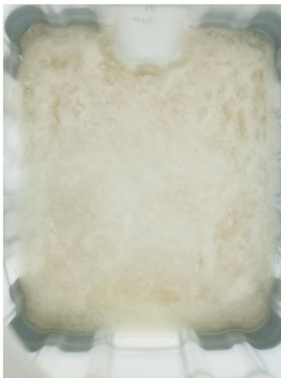
Figure 6.1. Solids Remaining in the Shipping Tote after Decanting to TK-01 in Test NB1.
