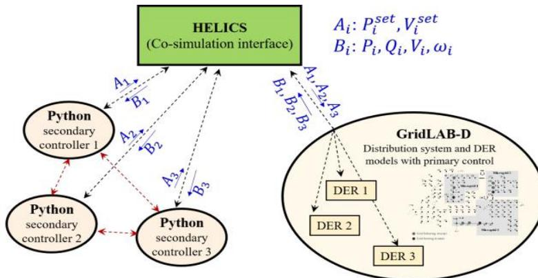
Fig. 2. Co-simulation platform for controlling of DERs in networked microgrids
