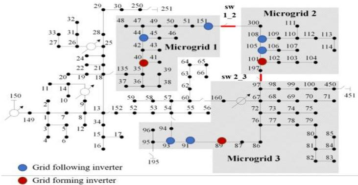
Fig. 1. A modified IEEE 123 test feeder to create a networked microgrid system
