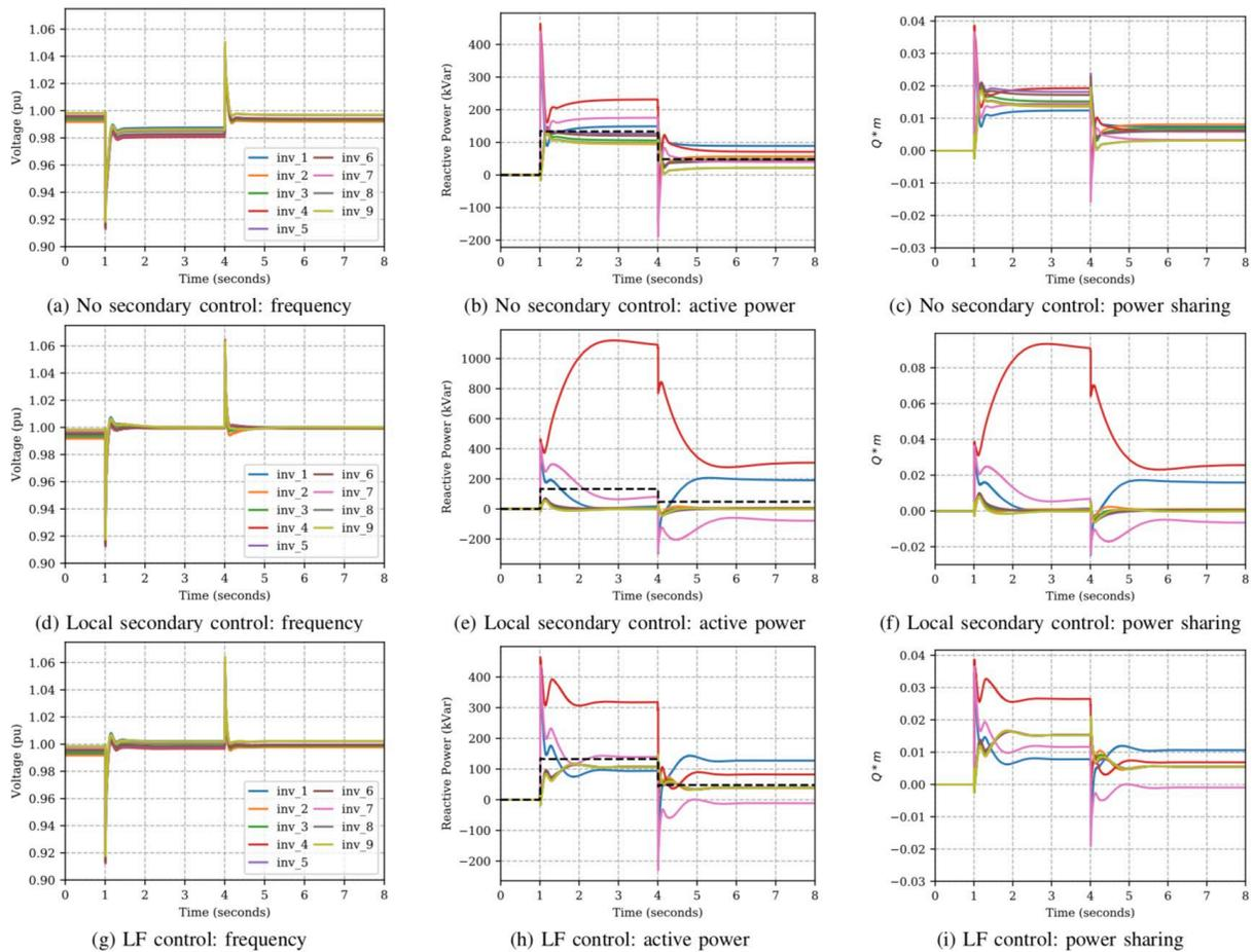
Fig. 4. Comparison of the voltage response by proposed control with no control and local control cases in the events of islanding and load disturbance
