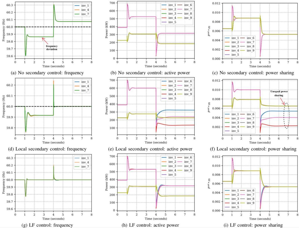
Fig. 3. Comparison of the frequency response of the proposed control with no control and local control cases in the events of islanding and load disturbance
