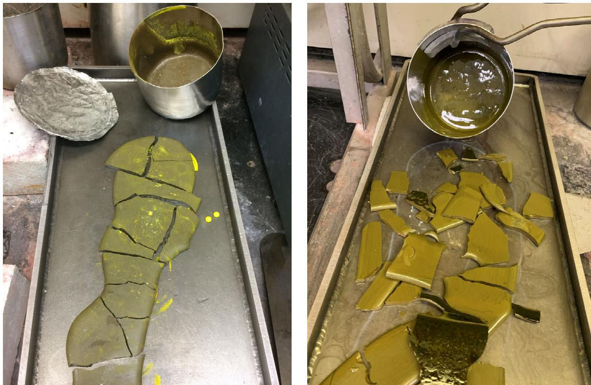
Figure 3-1. Images of LIC-02 after the first melt at 1200 °C (left) and the fourth and final melt at 1500 °C (right).
