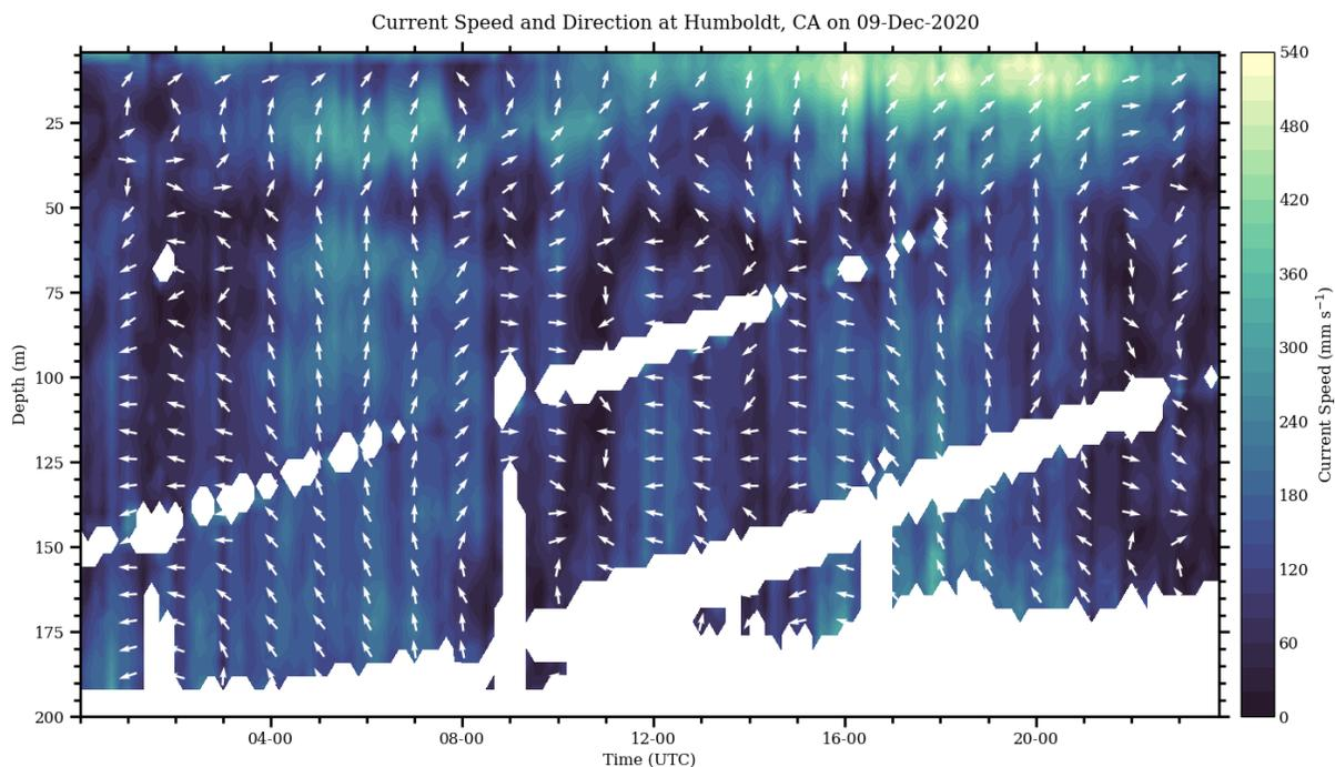
Figure 7. Time-Height Hovmöller diagram of Ocean current speed and direction at Humboldt on 9<sup>th</sup> December 2020. The data gaps represent poor signal to noise ratio of the ADCP measurements.
