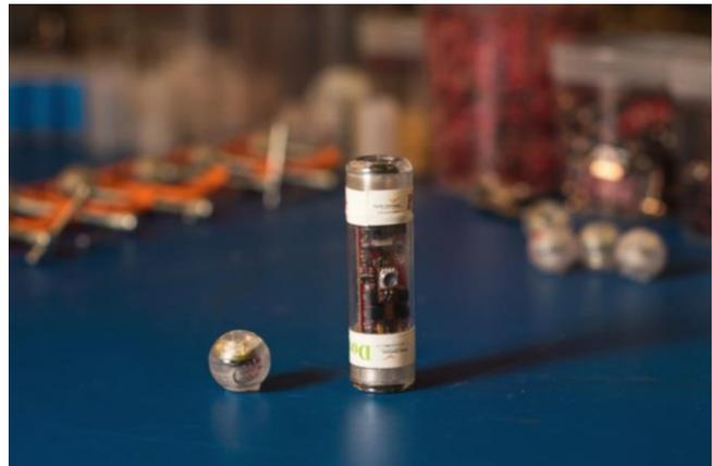
Figure 1. Sensor Fish (right) and Sensor Fish Mini (left).
