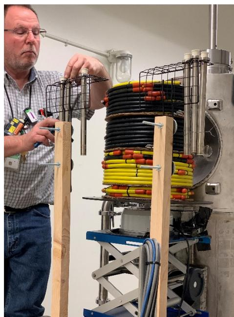
Figure 1 -Lignocellulose material mixtures in 5% hydrogen peroxide (stainless steel tubes) placed in the
