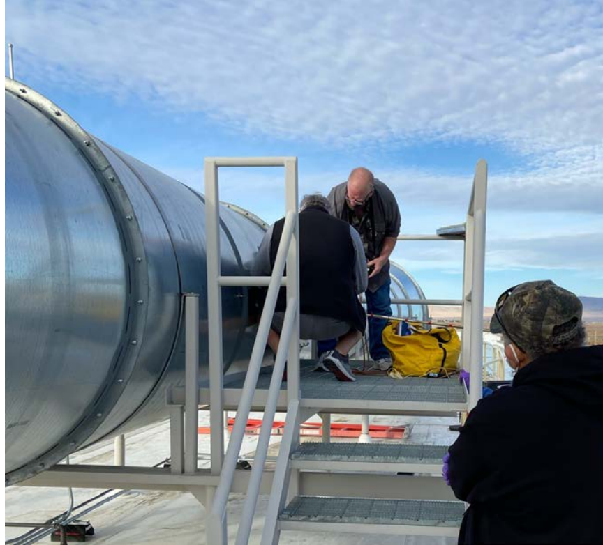
Figure 4. Photo of Staff Preparing for Traverse Measurements at the 3420 Stack Sampling Location.
