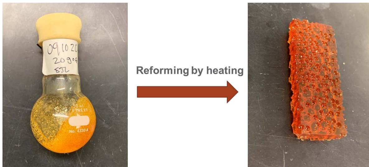
Figure 3. Benchtop demonstration of CO<sub>2</sub>-based vitrimer. Vitrimer (malleable thermoset) is formed/cured in a reaction flask shown on the left and reformed into a bar shape upon heating.
