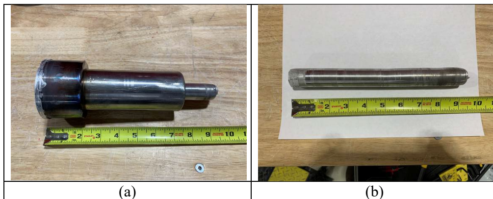
Fig. 4 (a) 1.0" dia extrudate contained within the extrusion die, (b) actual 1" dia. extrudate
