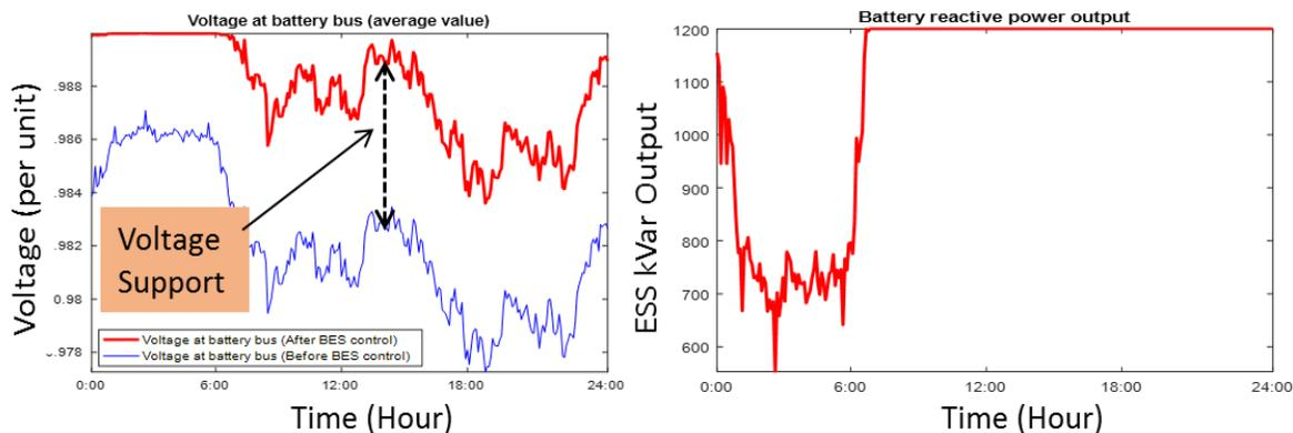
Figure 4.17. Voltage Profile at BESS Bus (Left); Reactive Power from BESS Inverters (Right)
