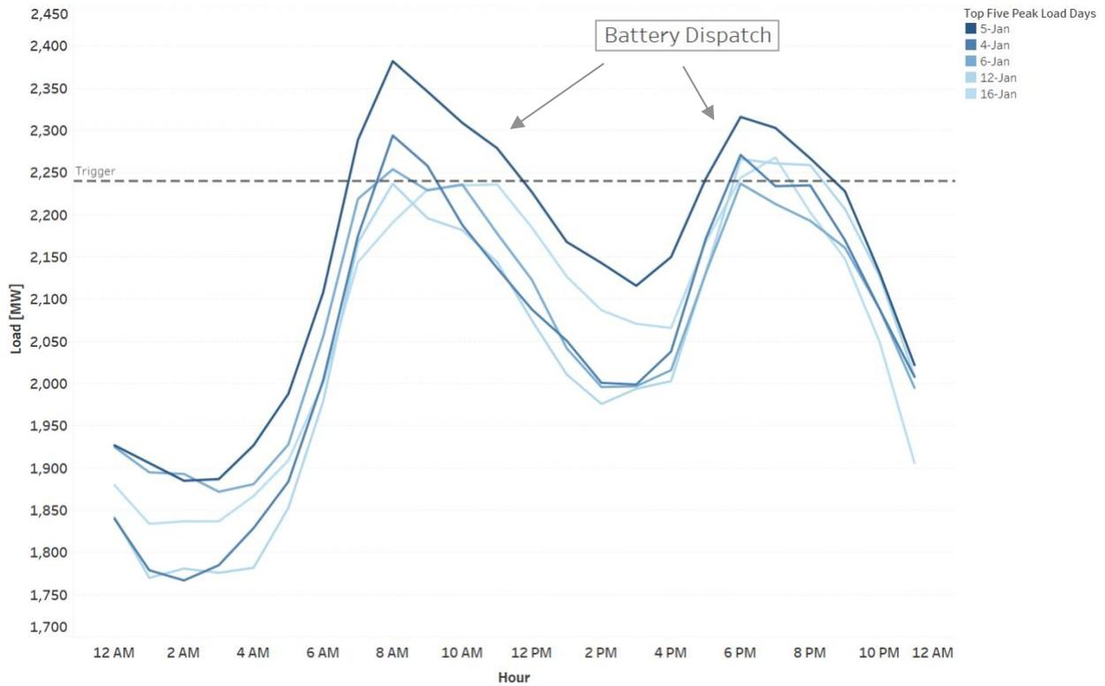
Figure 4.4. Example of Top Five Peak Load Days and Battery Dispatch for Capacity Benefit
