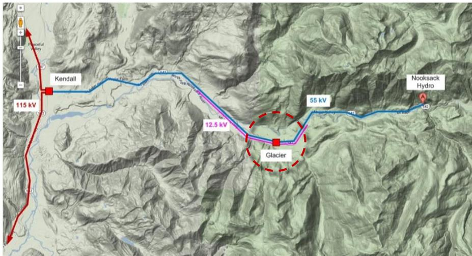
Figure 2.1. Glacier Location on the 55 kV Transmission Line
