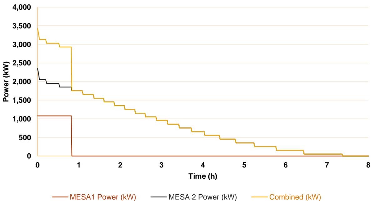
Figure 4.9 Maximum Output of MESA 1 and MESA 2 Within Capacity Period with 95% Confidence
