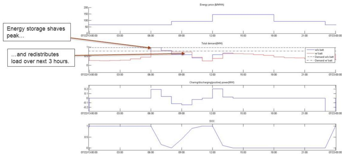
Figure 3.3. Base Load and Battery Operation for an Illustrative Day
