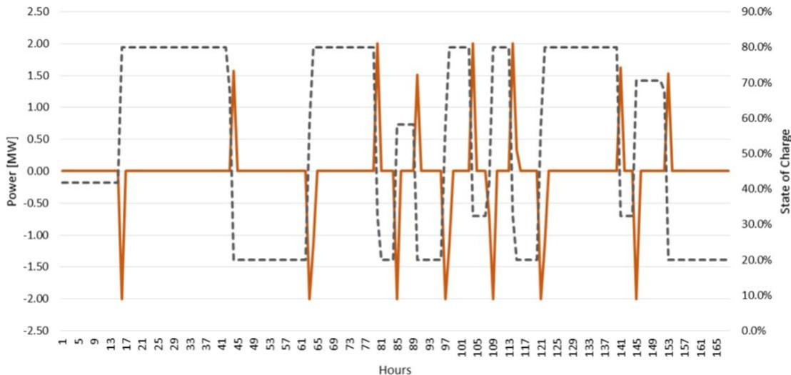
Figure 4.2. Arbitrage Duty Cycles of Battery by Hour
