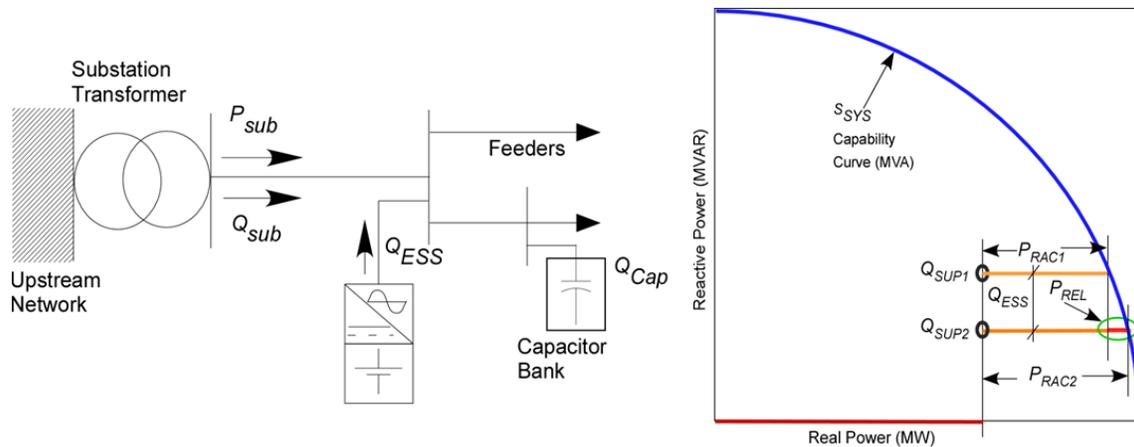
Figure 4.20. Release of Upstream Network Capacity in Terms of AC System Capability
