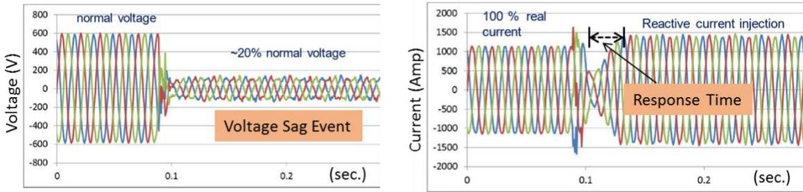
Figure 4.16. Voltage Waveforms During a Voltage Sag Event
