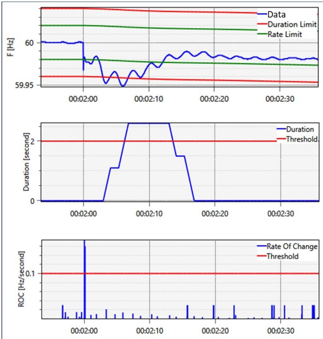
Figure 2-6. Screen capture from Archive Walker showing a frequency event (top) detected by both the duration-based detector (middle) and the detector based on rate-of-change (bottom).
