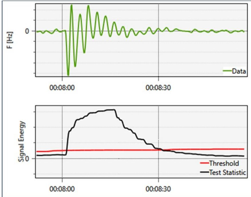
Figure 2-4. Screen capture from Archive Walker showing a ringdown (top) along with the RMS energy and threshold used to detect it (bottom).
