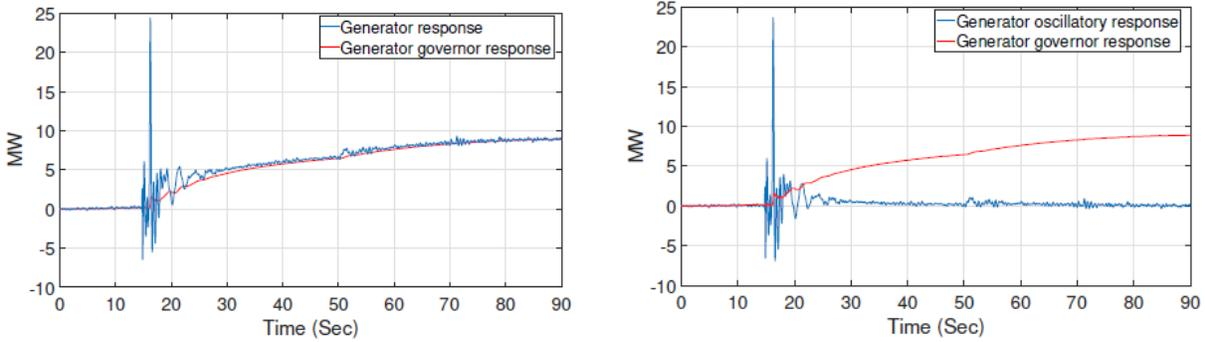
Figure 5-19. Separated governor and oscillatory response using high-pass filter
