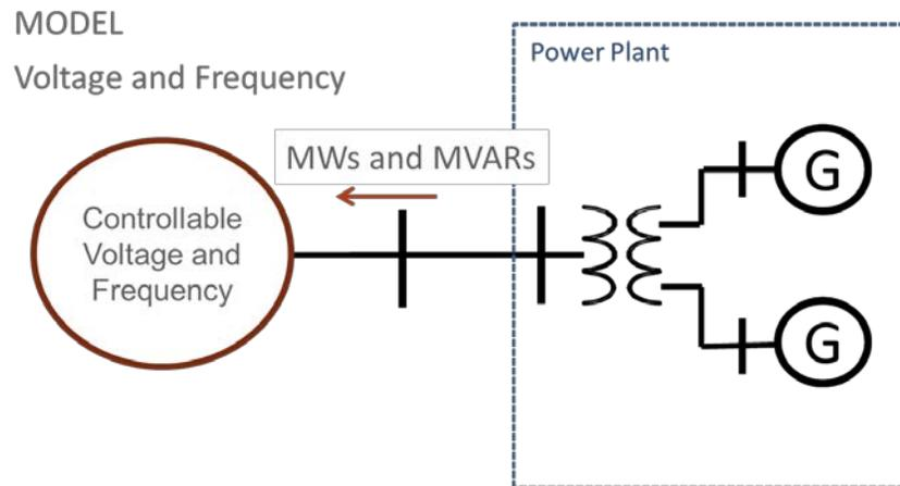
Figure 5-2. Illustration of the disturbance recordings-based power plant model validation
