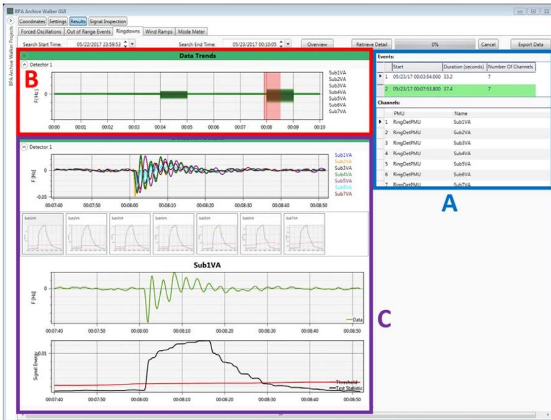
Figure 2-2. Screen capture of Archive Walker with results displayed in (A) a table of events, (B) a plot of the input signals' extrema, and (C) plots detailing the detector's operation.
