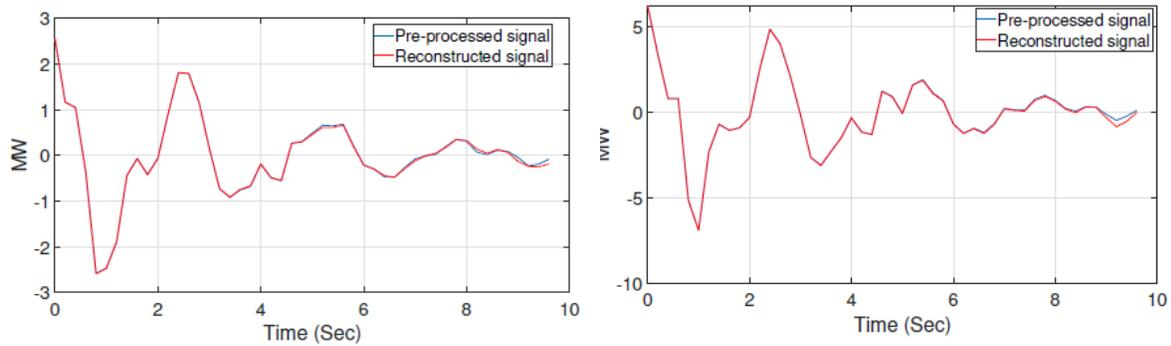
Figure 5-23. Illustration of the model order selection by comparing pre-processed and signal reconstructed by using mode and mode-shape estimates for a. Actual response (model-order = 22 and goodness of fit = 0.96) and b. Model-based response (model-order = 22 and goodness of fit = 0.97)
