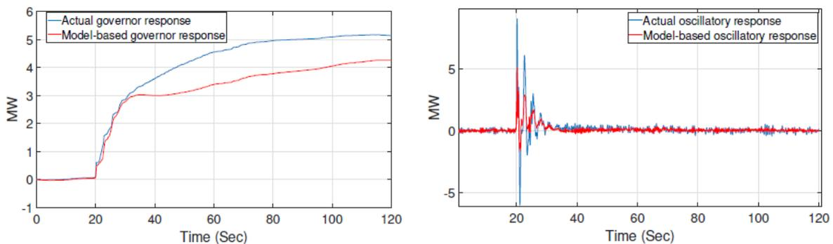
Figure 5-22. Generator governor (left) and oscillatory response (right) calculated using actual and model-based response
