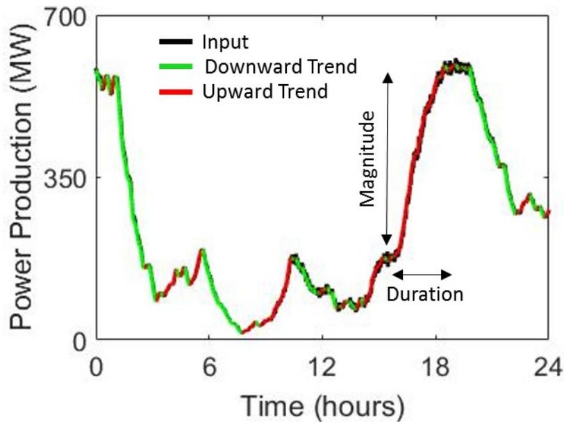
Figure 2-8. Example operation of the trend identifier within the wind ramp detector.
