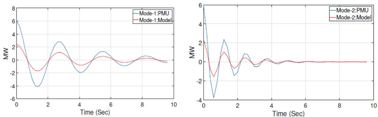
Figure 5-24. Comparison of contribution of selected modes to the magnitude component of oscillatory response of actual and model-based response – a. Mode-1 (left) b. Mode-2 (right)
