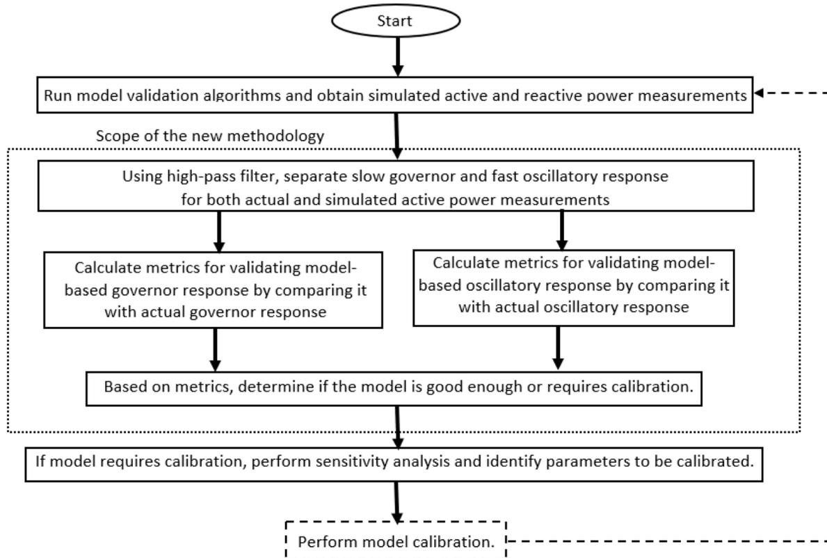
Figure 5-18. Flowchart for the methodology for quantifying model validation results
