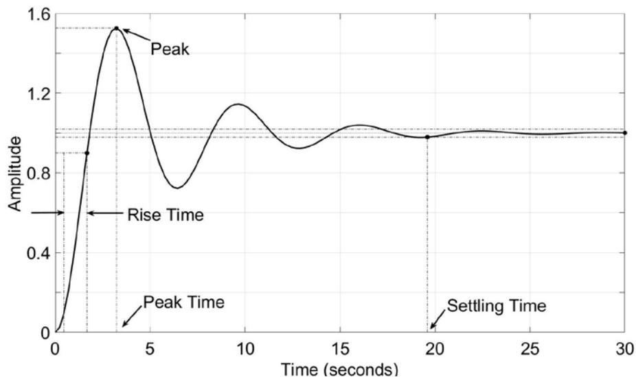
Figure 5-20. Step-response characteristics of a system
