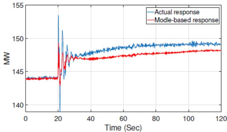
Figure 5-21. PMU measurements recorded at the Point of Interconnection, and model-based response of the generator obtained using PPMV tool
