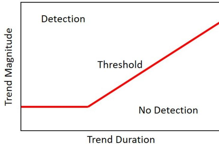
Figure 2-9. Detection threshold utilized in the wind ramp detector.
