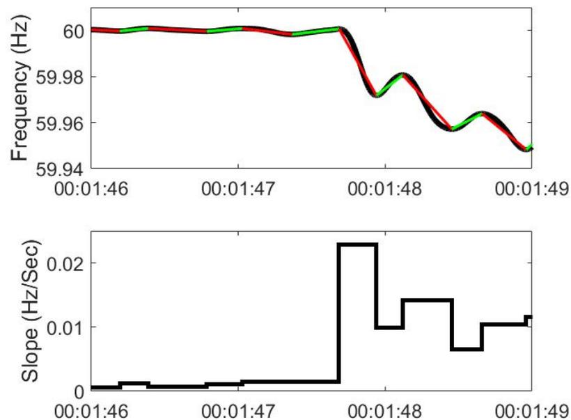
Figure 2-5. Example operation of the out-of-range event detector's rate-of-change stage. The slopes in the bottom plot correspond to the red and green lines connecting extrema of the input signal in the top plot.
