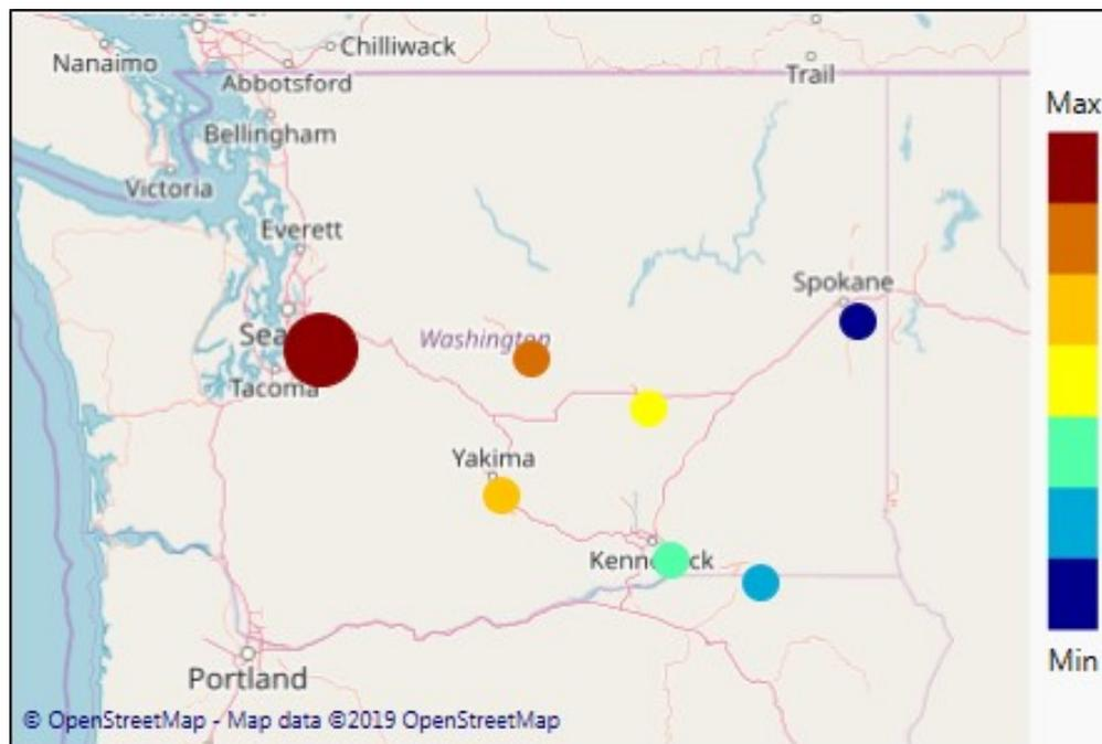
Figure 2-7. Screen capture from Archive Walker displaying a forced oscillation's amplitude at several measurement locations.
