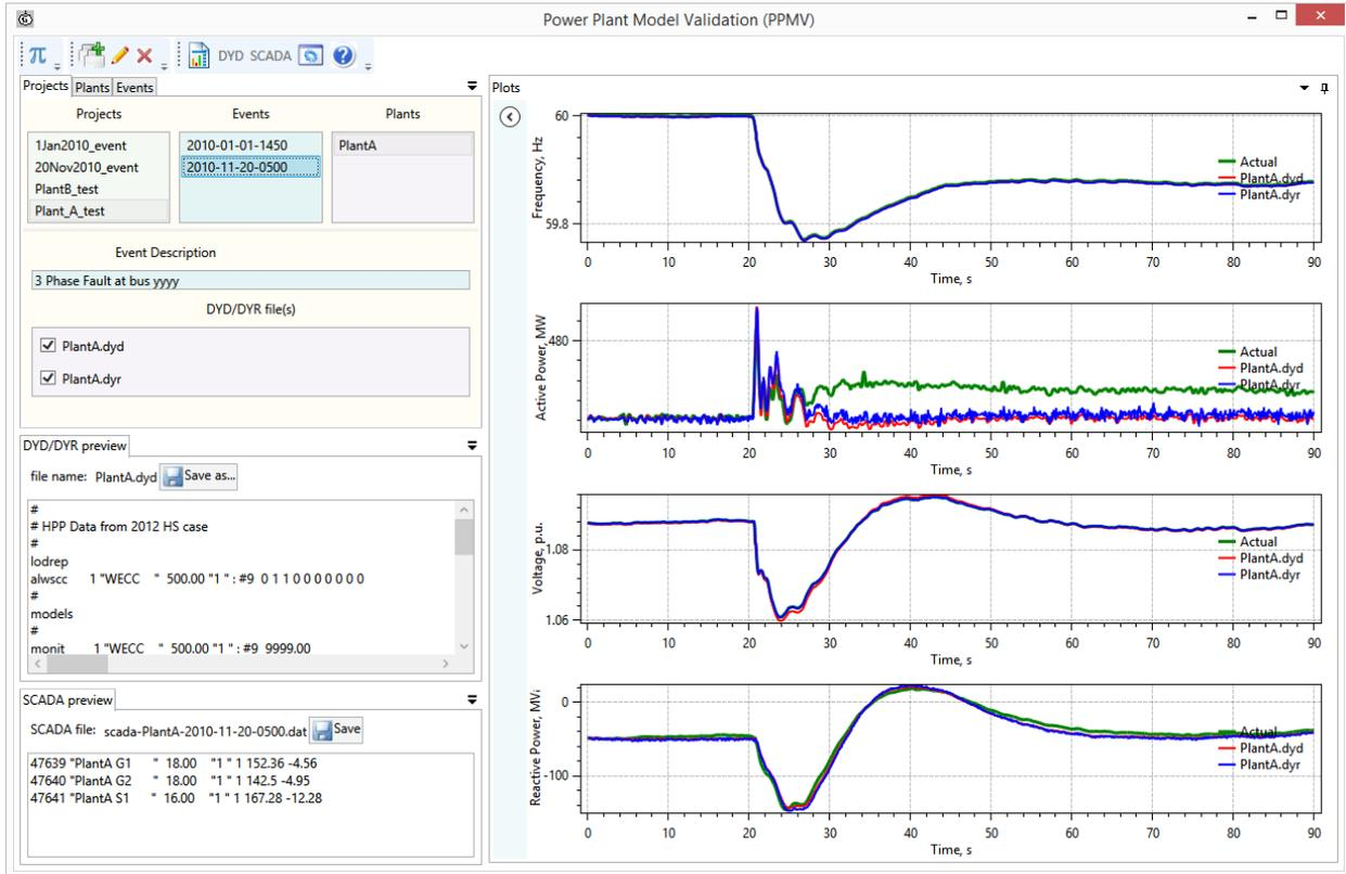
Figure 5-3. GUI of the PPMV tool developed by PNNL and BPA
