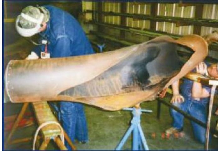
Figure 3-9 Ruptured elbow caused by FAC. (Ahmed 2012)
