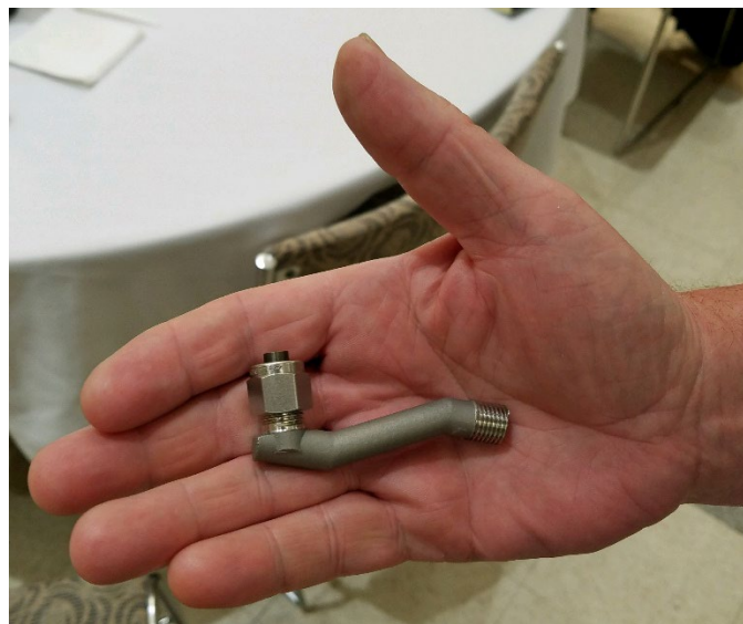
Figure 2-6 Miniature nozzle for confined spaces as small as 1.5 in. (38 mm) (PNNL photo).
