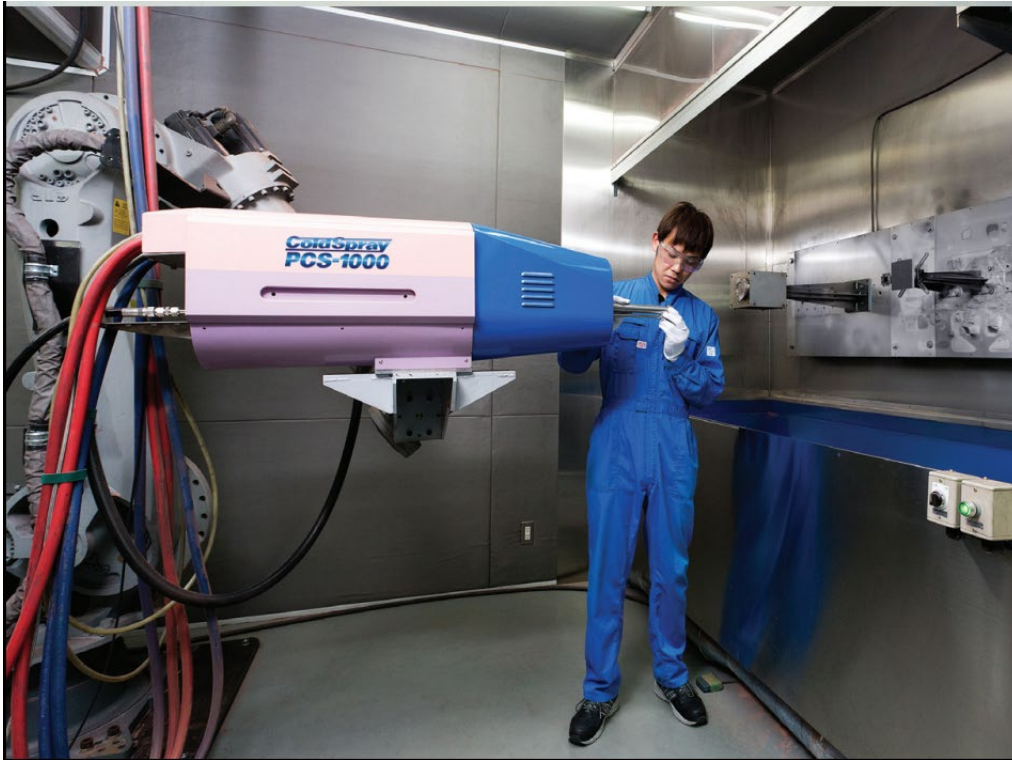
Figure 2-4 High pressure stationary industrial CS equipment for factory CS of high melt temperature materials such as MCrAlY (a family of thermal and corrosion barrier coatings where M = Co, Ni or Co/Ni), Ti6Al4V, Inconel, and SS (Plasma Giken 2018). In general, stationary equipment with large CS guns offer improved properties and economics compared to portable equipment for high melt temperature alloys.
