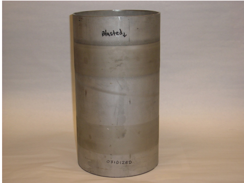
Figure 3-7 Ni coating on a 6 in. Schedule 10 SS304 pipe section. Two layers of Ni approximately 0.020 in. thick total. Each band is 3 in. wide. The surface was grit blasted for the upper band and was oxidized for the lower band. The yield for Ni deposited with this process was measured at 115 ksi (sample courtesy of ARL).
