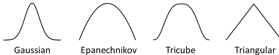
Figure 3. Example kernels for use with the kernel smoothing algorithm.
