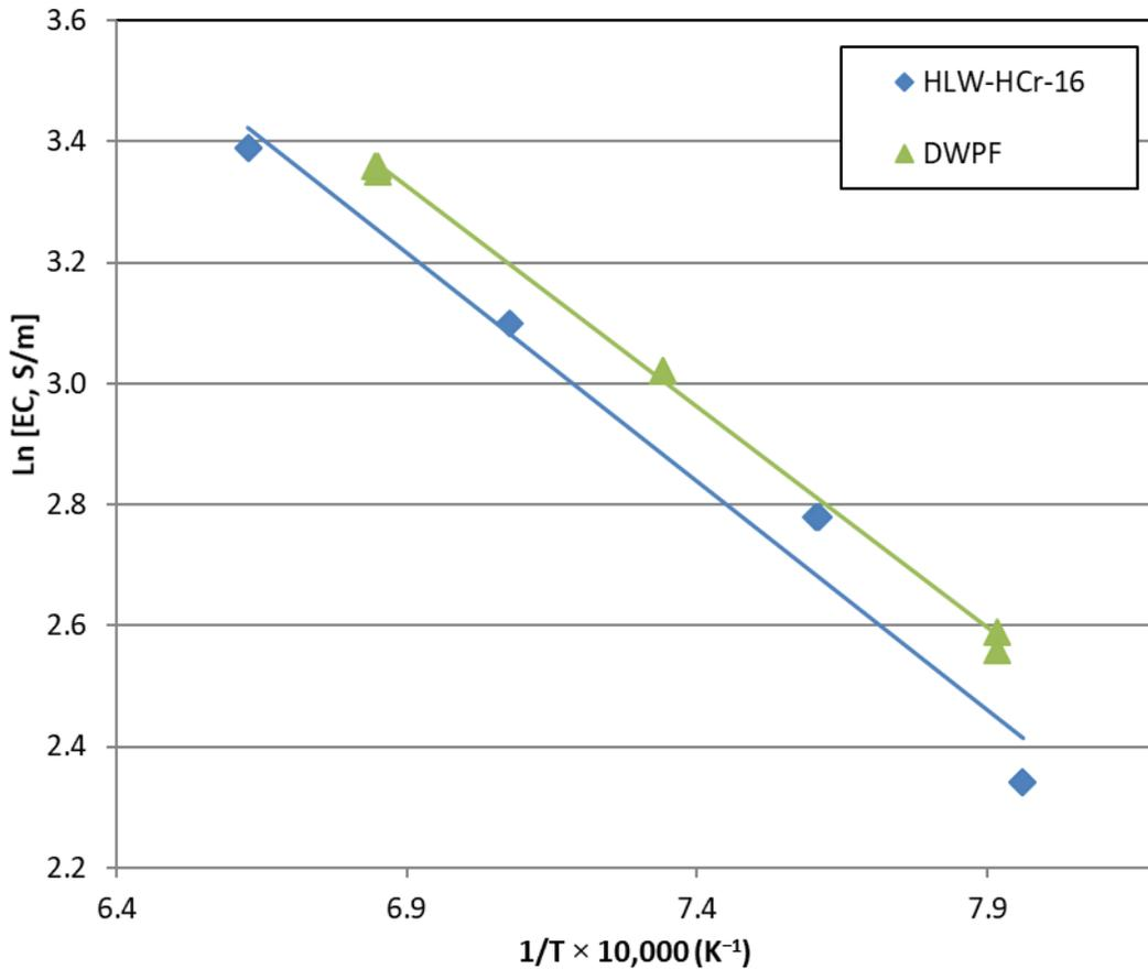
Figure 6.7. Electrical Conductivity of HLW-HCr-16 Glass and DWPF Reference Glass
