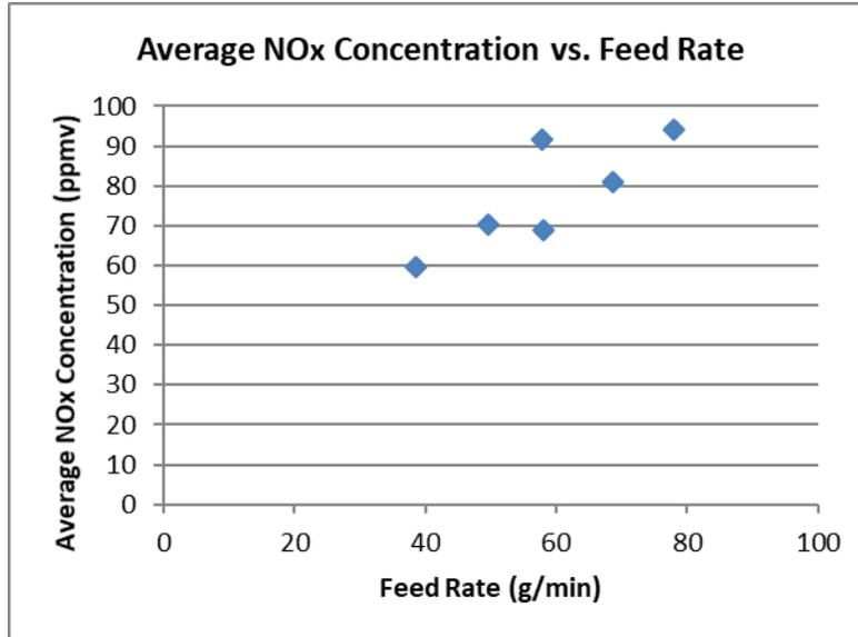
Figure 8.4. Feed Rate vs. NO<sub>x</sub> Concentration in RSM Offgas
