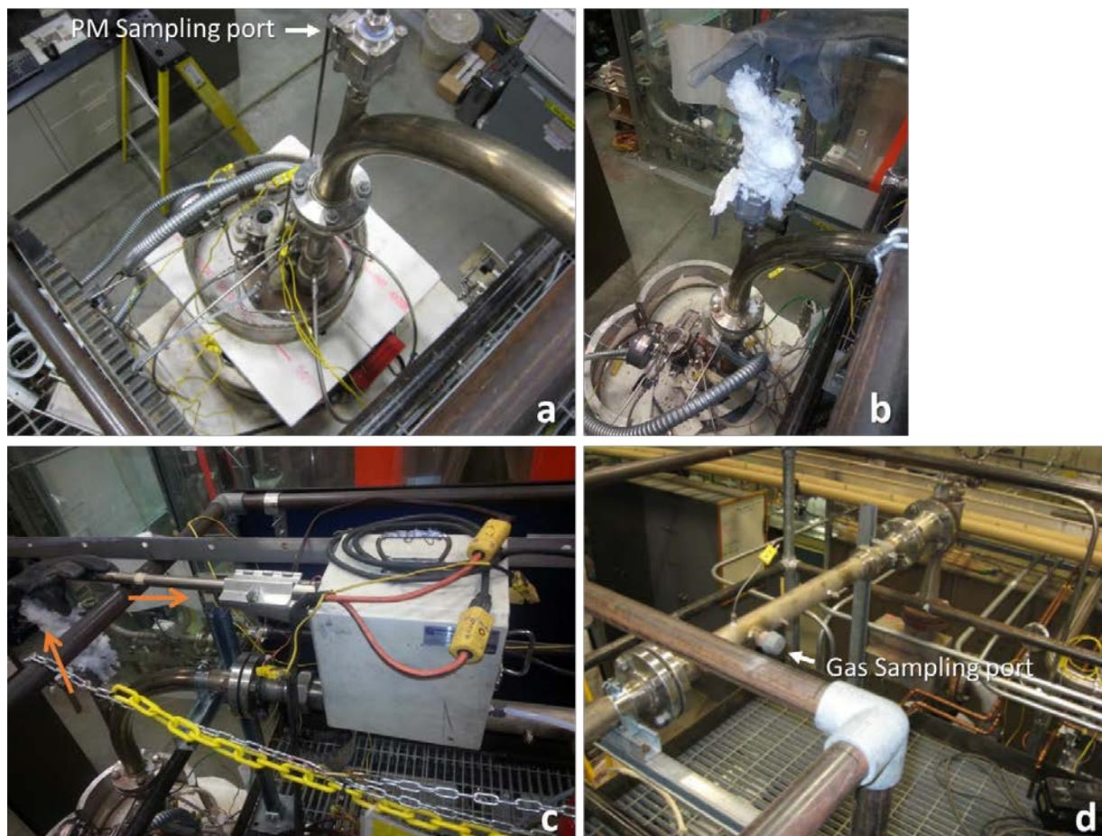
Figure 8.1. Sampling Locations. (a) PM sampling port on top of the RSM (next to the 90° bend in exhaust pipe); (b) PM sampling port with PM filter installed; (c) PM filter, the orange arrows mark the PM sampling Line, with the main exhaust pipe on the bottom; (d) gas sampling port in horizontal section of exhaust pipe
