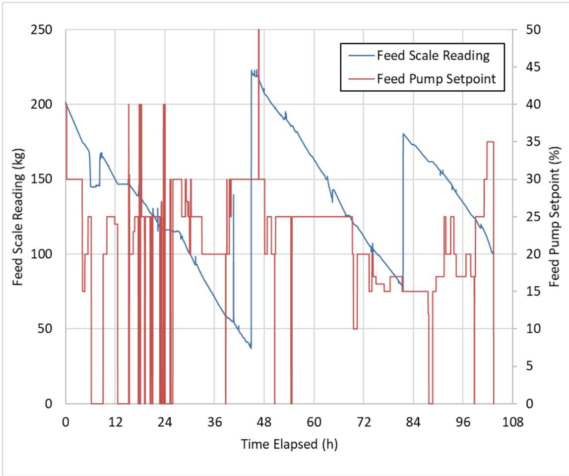
Figure C.1. Simulant Feed Pump Set Point and Balance Reading
