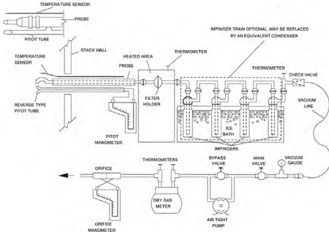
Figure 8.6. EPA Method 5 Particulate Sample Train Diagram
