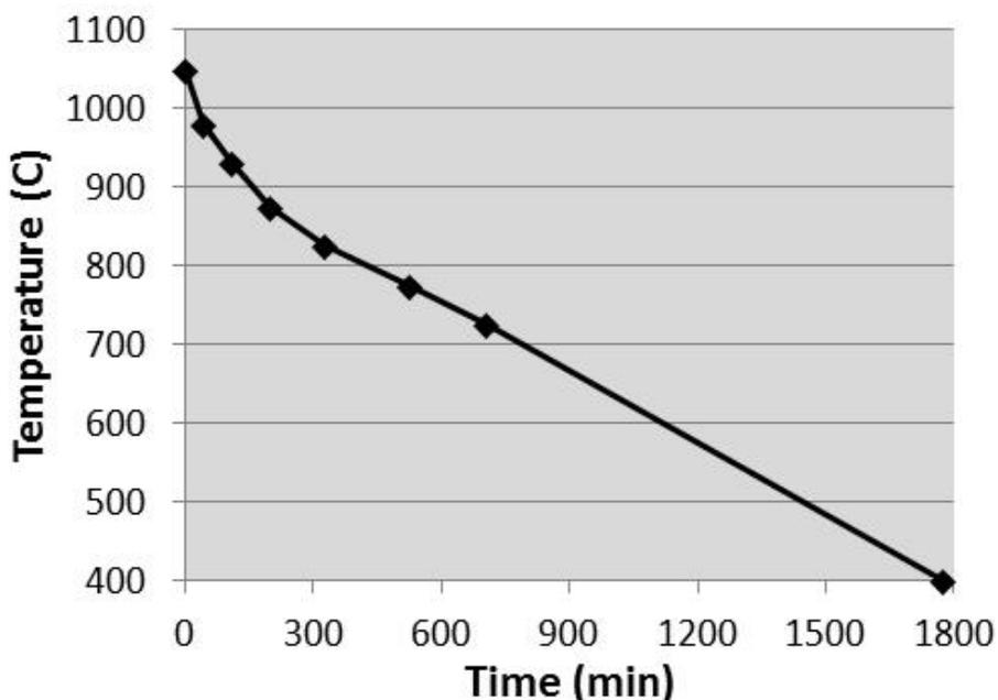
Figure 6.1. Graph of CCC Heat Treatments of HLW Glass
