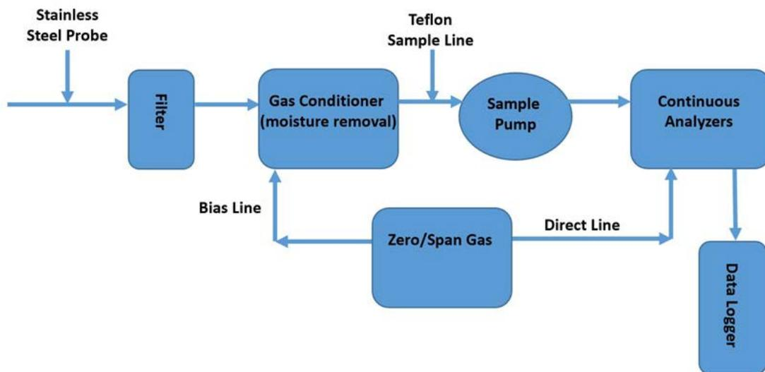
Figure 8.3. EPA Methods 3A, 7E, and 10 Analyzer Sample System Diagram
