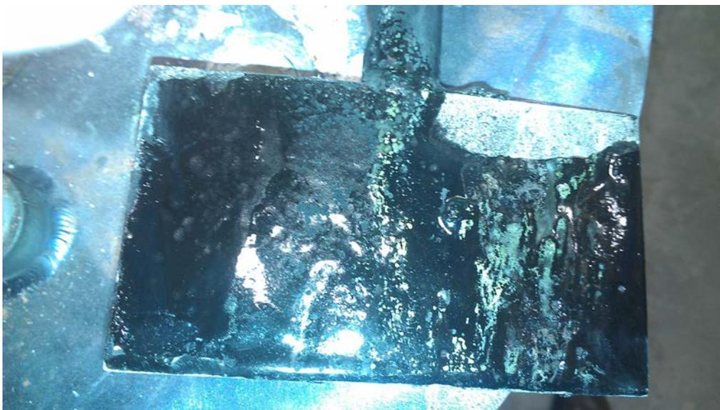
Figure 4.4. Melter Electrode Pulled from the Glass Melt
