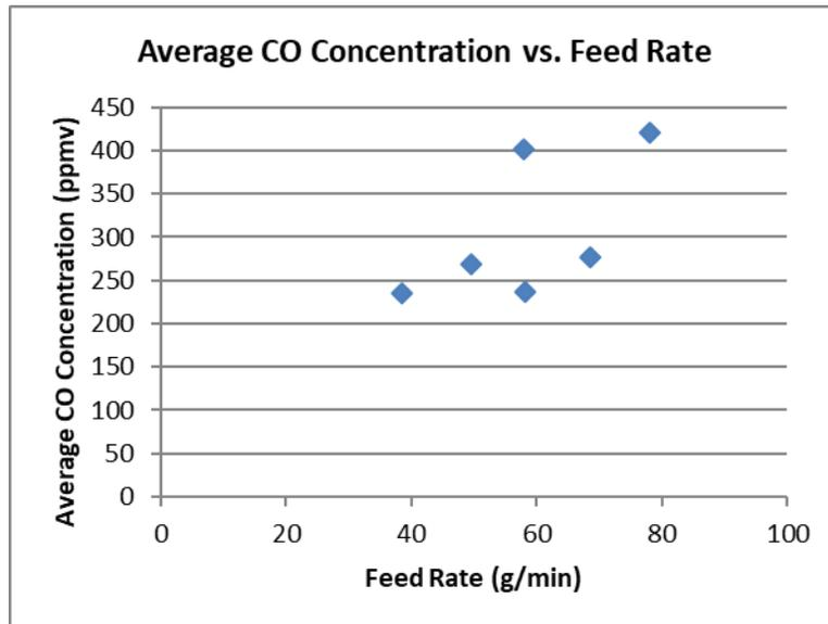
Figure 8.5. Feed Rate vs. CO Concentration in RSM Offgas
