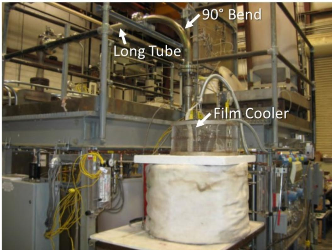
Figure 4.6. Areas in Offgas Line from which Samples of Deposit Material Were Collected
