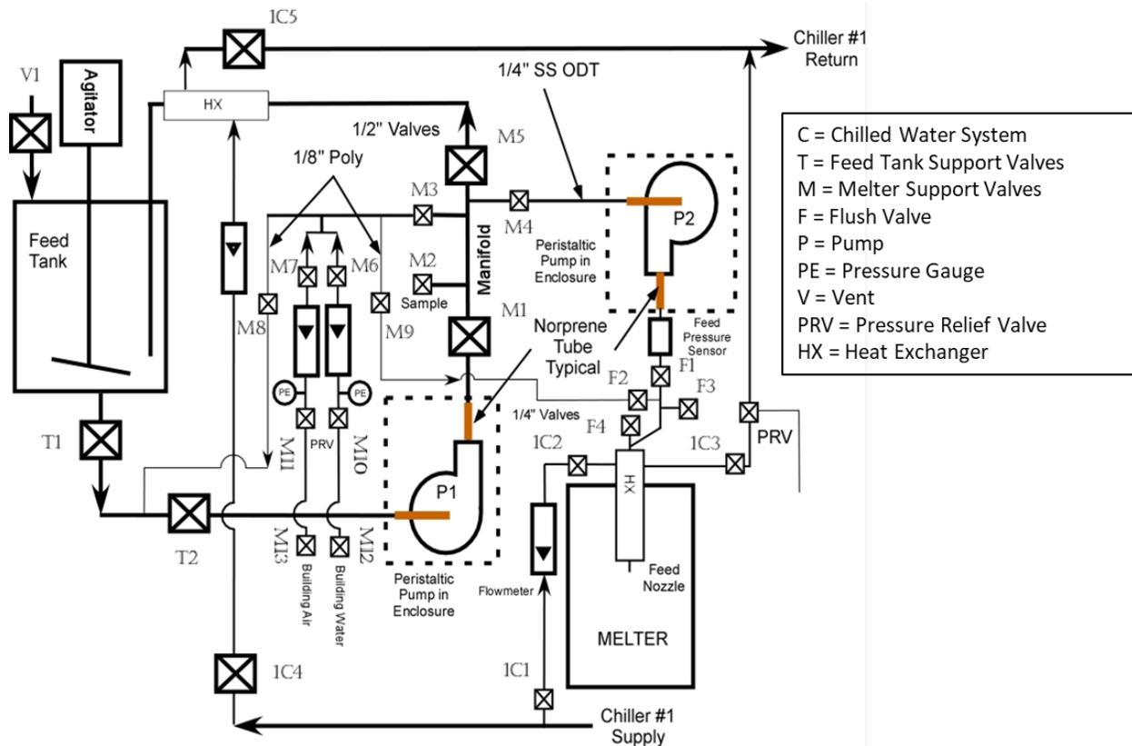
Figure 2.2. RSM Feed System Diagram
