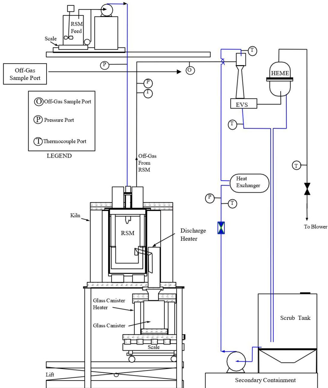
Figure 2.1. Research-Scale Melter Configuration
