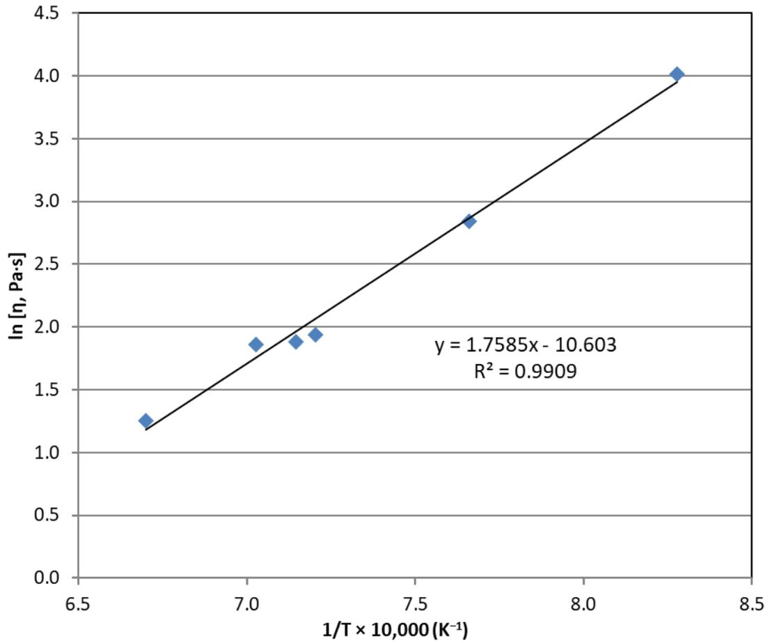
Figure 6.8. Viscosity of HLW-HCr-16 Glass as a Function of Temperature (Sample RSM-EWG8-044)
