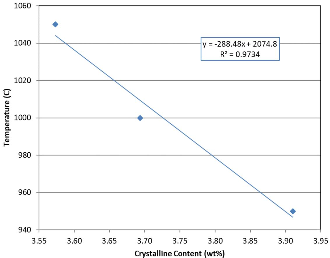
Figure 6.6. Temperature vs. Spinel Content for HLW-HCr-16 Glass Melted at PNNL
