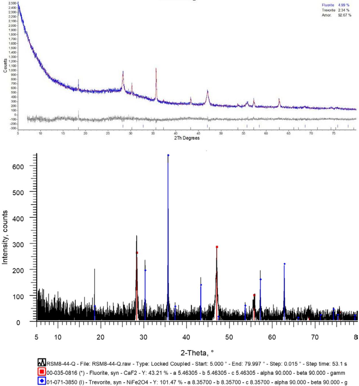
Figure 6.4. XRD Pattern of Quenched Glass (sample ID RSM-EWG8-044) Examined microscopically in Figure 6.2
