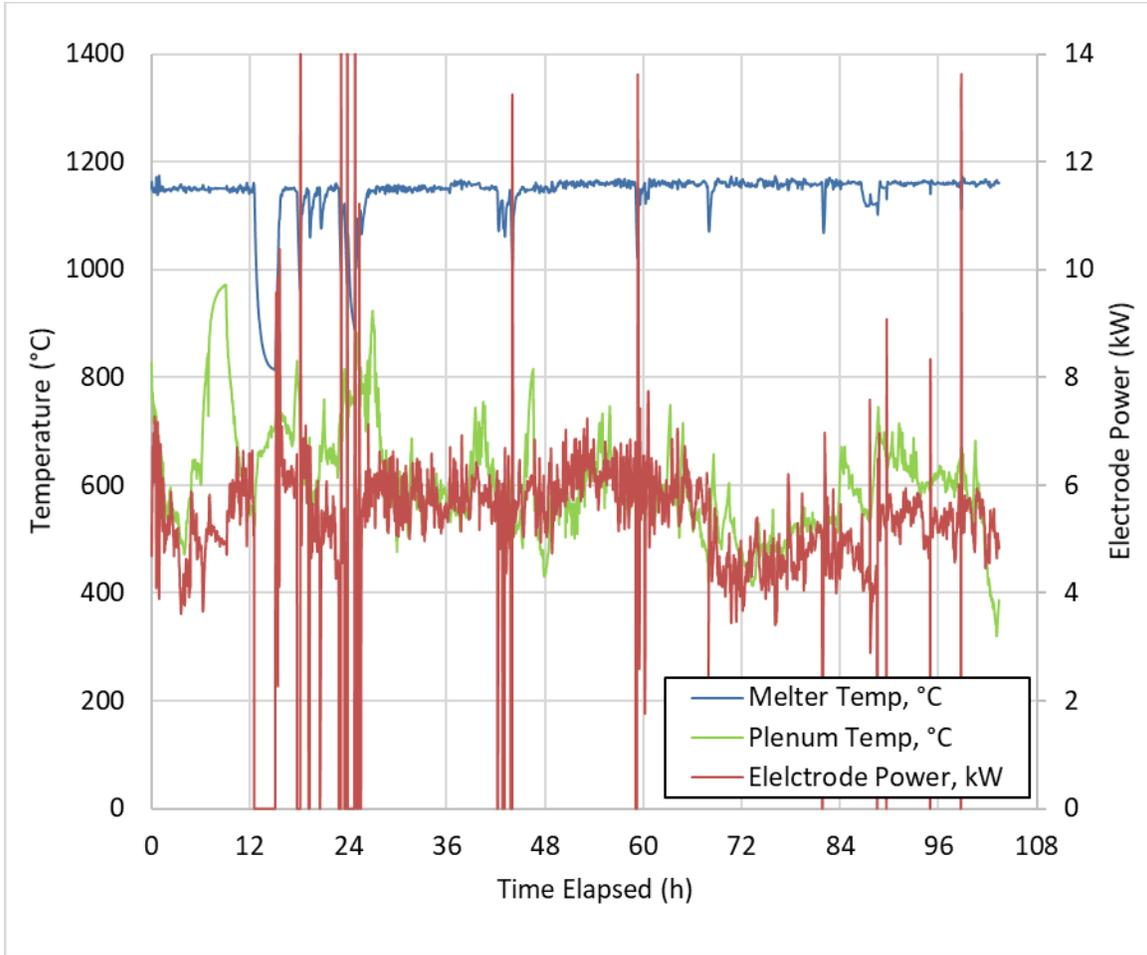
Figure C.3. Melter and Plenum Temperatures and Electrode Power
