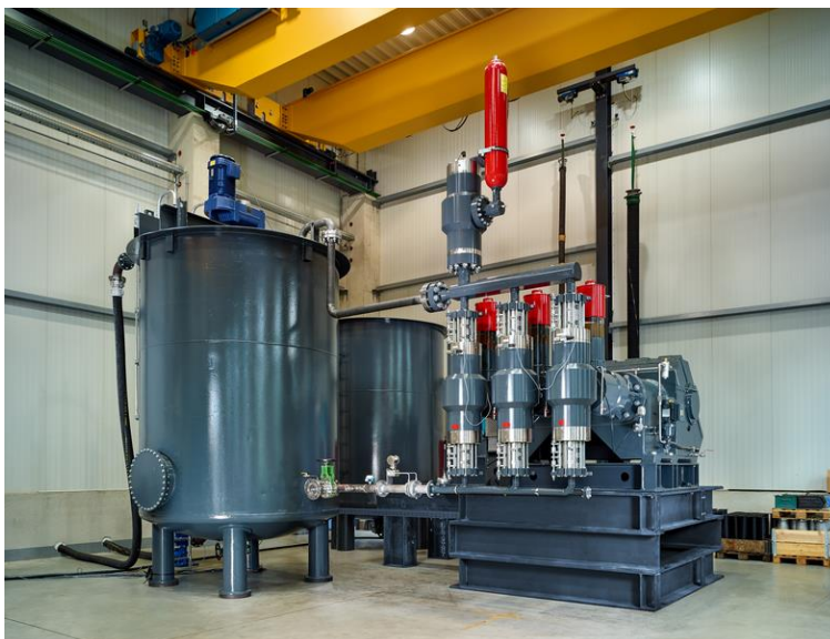
Figure 1. FELUWA Pumpen new slurry pump test system available for customer feed evaluation. Source: FELUWA Pumpen GmbH
