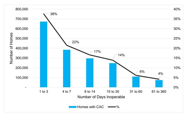
Figure 11. Duration of equipment failure for U.S. single-family homes with CACs
