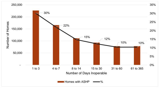
Figure 12. Duration of equipment failure for U.S. single-family homes with ASHPs
